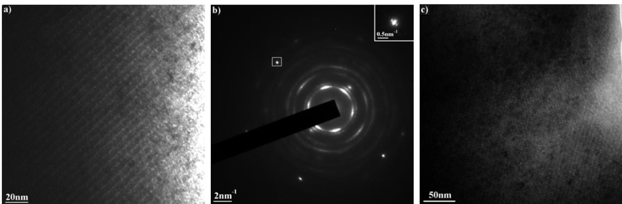
Figure 3 : a) Bright field image of the bubble superlattice found in the U(Mo) particles. b) Corresponding diffraction pattern, where the inset shows an enlarged image of the (222) reflection from the [-211] zone indicated by the square. c) Observation of the bubble superlattice in an adjacent grain at the same position. Here, the orientation is such that individual bubbles can be more clearly observed.
