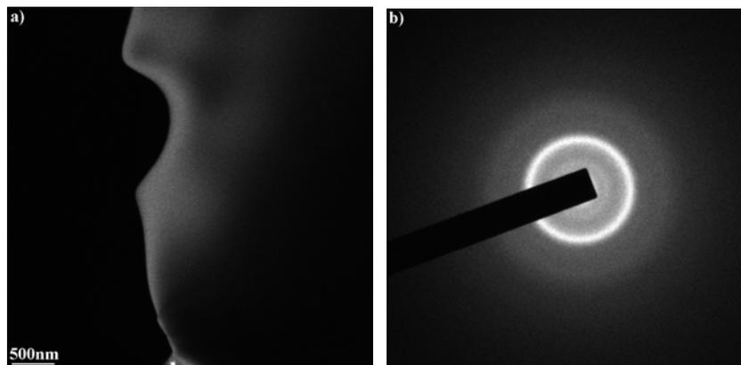
Figure 1: a) Dark field image of the interaction layer with b) the diffraction pattern, demonstrating its fully amorphous character.
