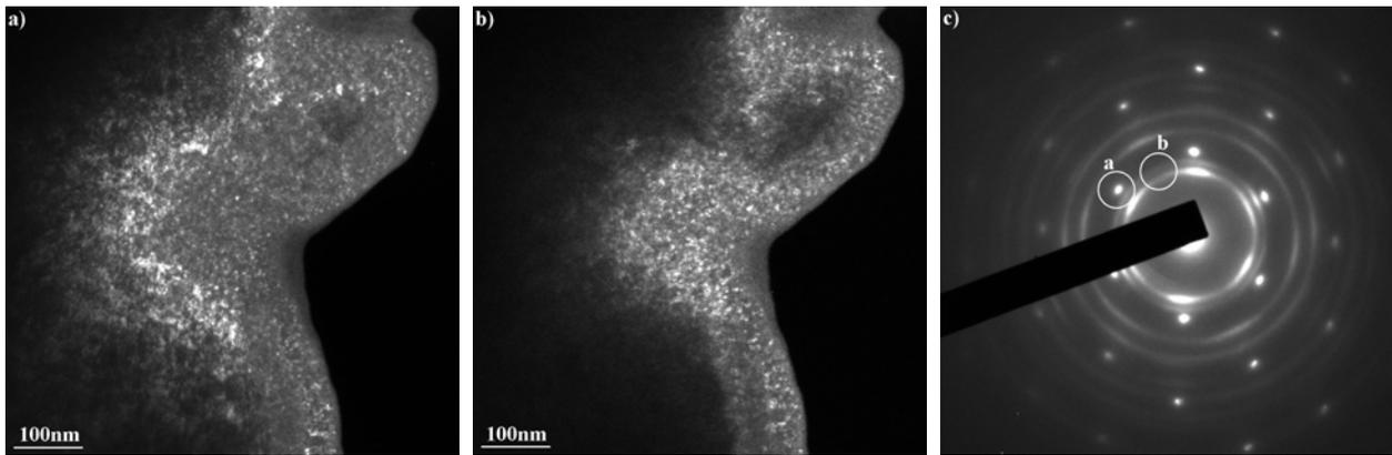
Figure 2 : Dark field images and the corresponding diffraction pattern of a transparent region in the U(Mo) fuel, taken using a) a (110) U(Mo) reflection and b) with part of the UO<sub>2</sub> diffraction ring as indicated by the white circles in the diffraction pattern in c).
