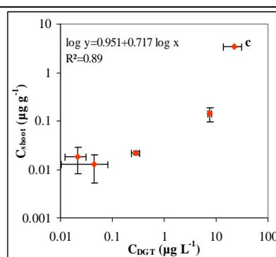
Fig. 1b: Relation between  $C_{\text{DGT}}$  and U concentrations in ryegrass shoots for soils with different contamination history
