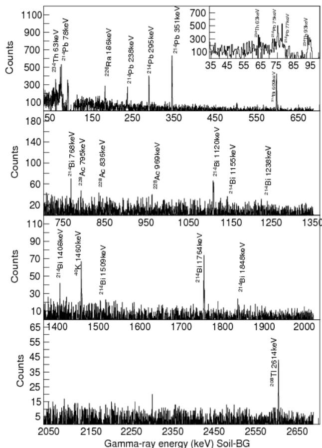
Figure 6: Background-subtracted gamma-ray spectrum associated with soil sample 228 with lines from the  $^{238}\text{U}$  decay series clearly identified spread on four panels.
