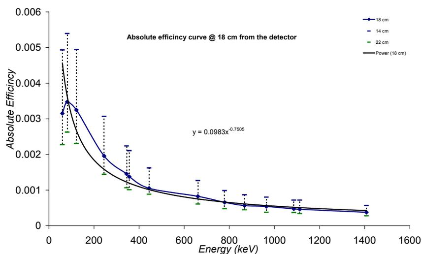
**Figure 4: Absolute Efficiency calibration using peaks from standard  $^{152}\text{Eu}$ ,  $^{137}\text{Cs}$ ,  $^{241}\text{Am}$  and  $^{133}\text{Ba}$  sealed point sources which were placed at distances of 14, 18, 22 cm from the front face of the HpGe detector.**
