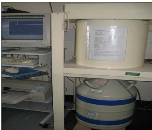
**Figure 3: a coaxial high purity Ge (HPGe) detector surrounded by lead shield of about 10 cm thickness.**
