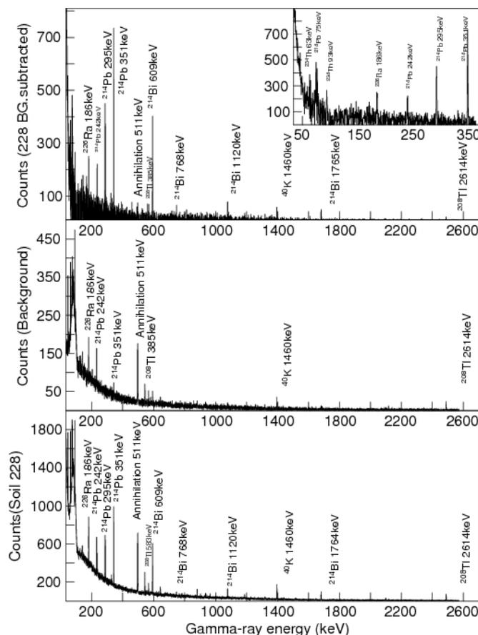
**Figure 5:(Lower panel) Raw  $\gamma$ -ray spectra of sample 228; (Central Panel) background spectrum accumulated in the absence of any source sample; (Upper Panel) background-subtracted gamma-ray spectrum associated with soil sample 228 with lines from the  $^{238}\text{U}$  decay series clearly identified.**
