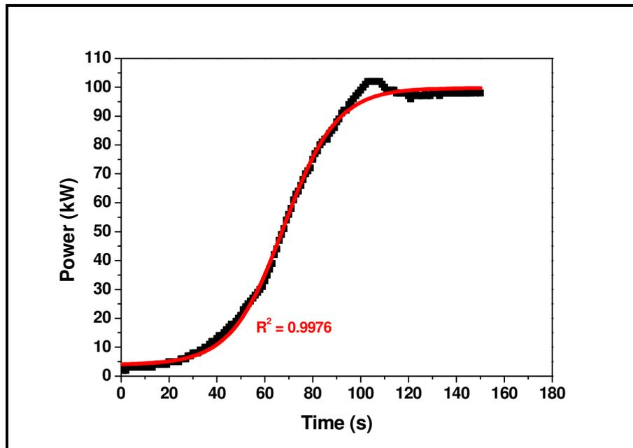
**Figure 5. Power evolution during IPR-R1 startup.
