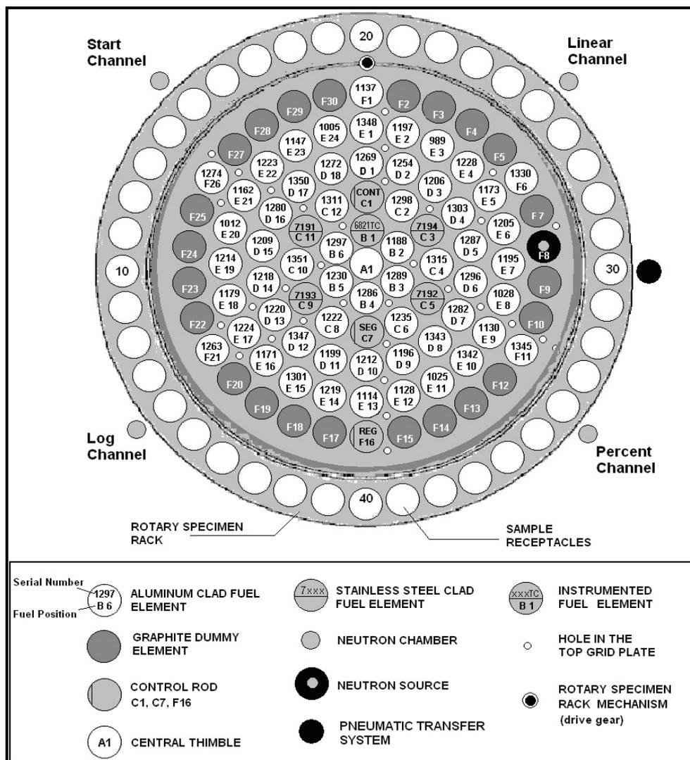
Figure 1. IPR-R1 TRIGA reactor core [3].
