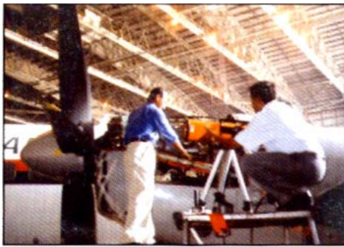
Radiographic testing of aircraft
