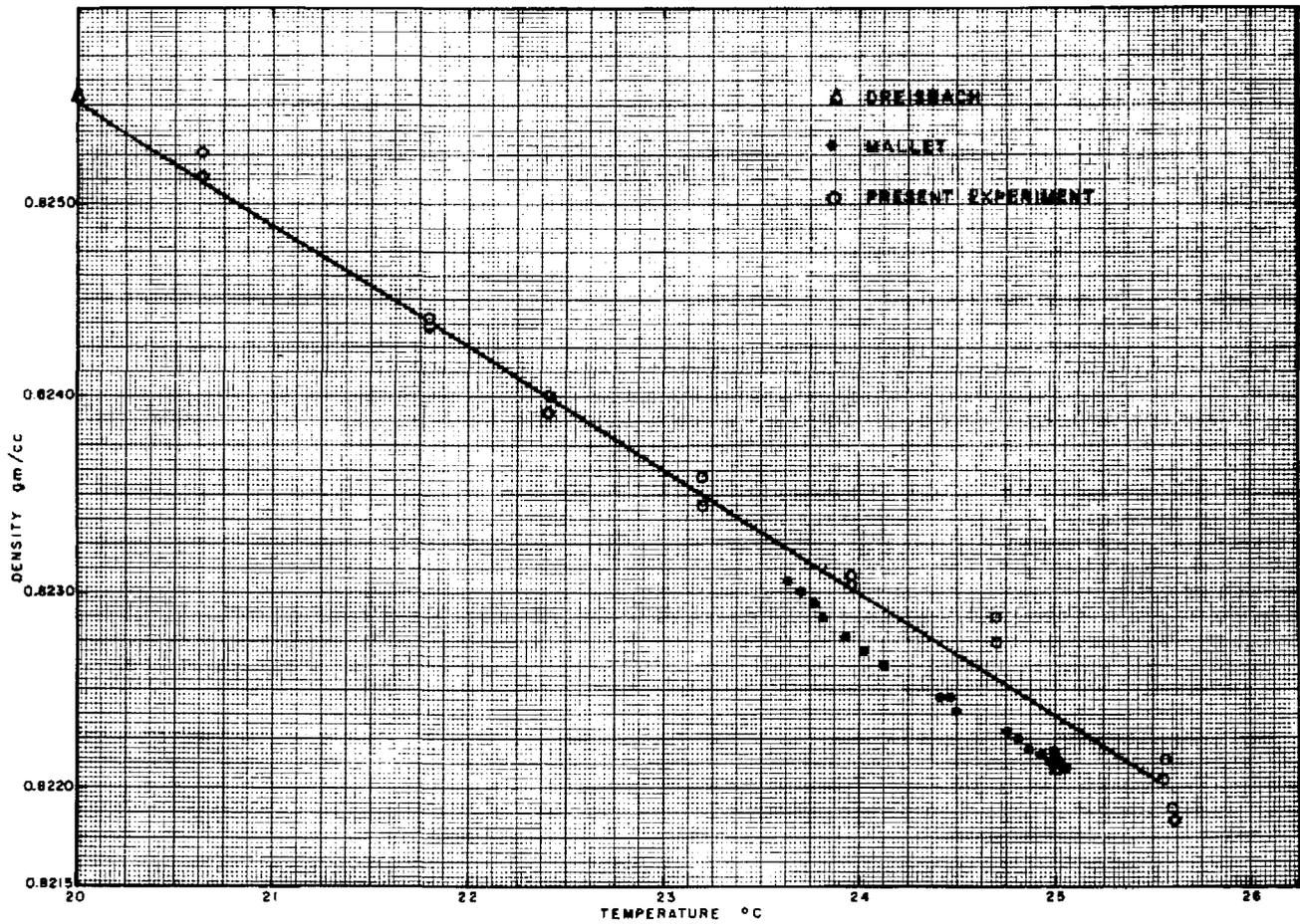
Figure 2: Density of n-octyl alcohol measured with a pycnometer.
