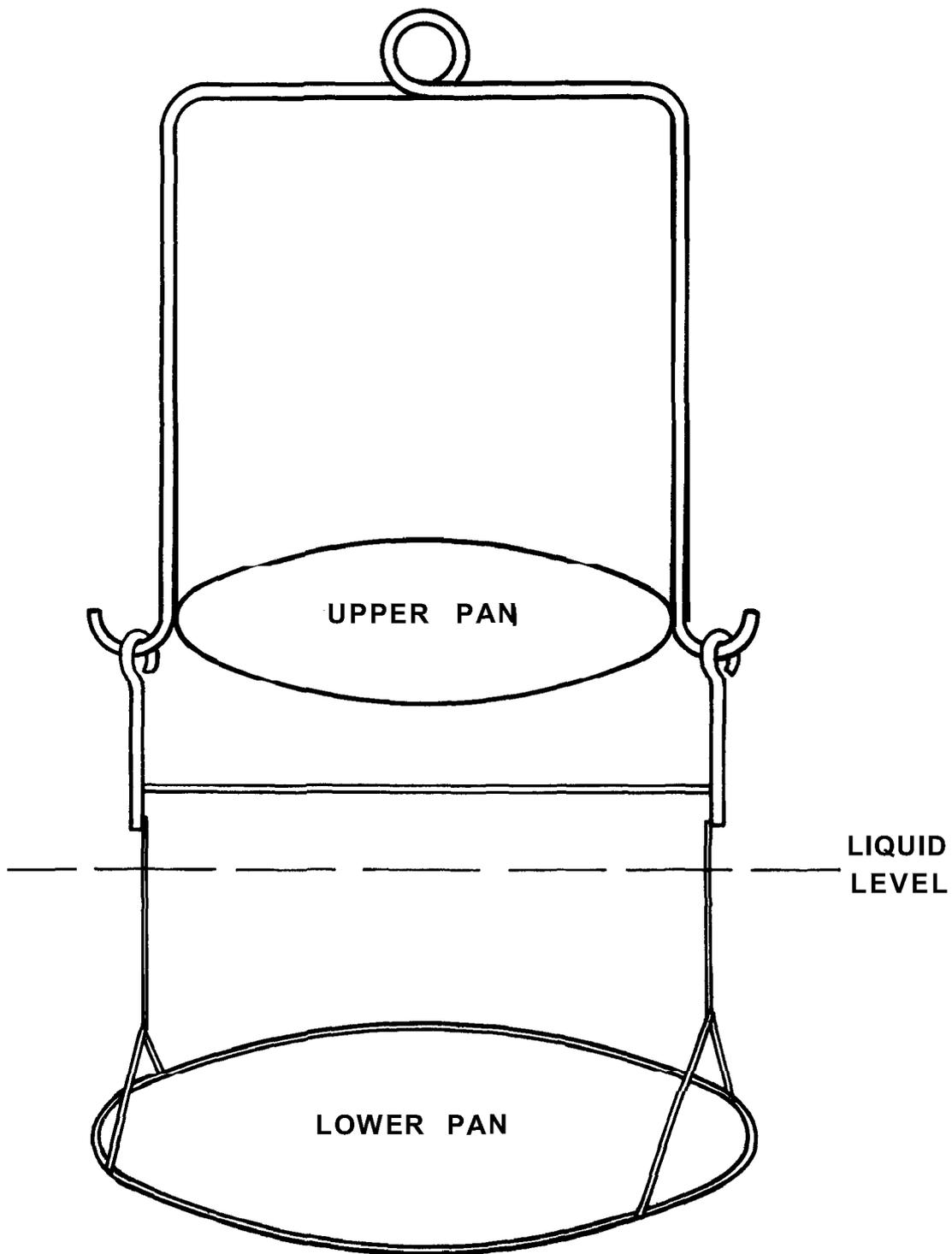
Figure 1: Balance pan assembly for density measurements.
