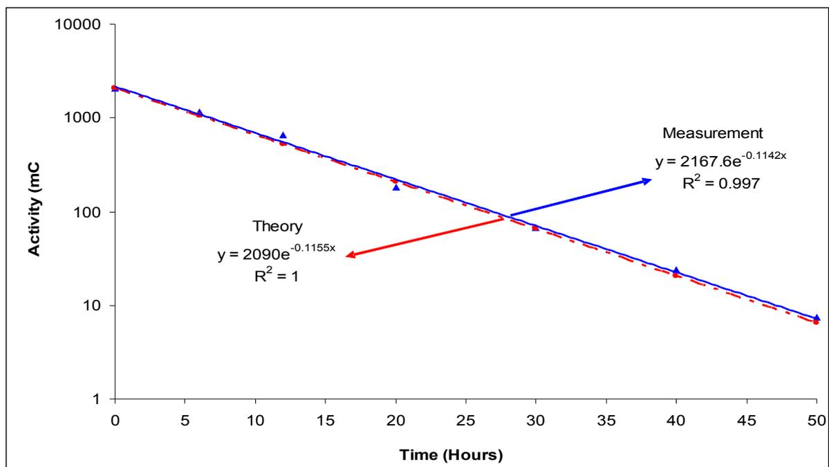
**Figure 6:** Linearity results using the decay method for CRC-15 beta dose calibrator.
