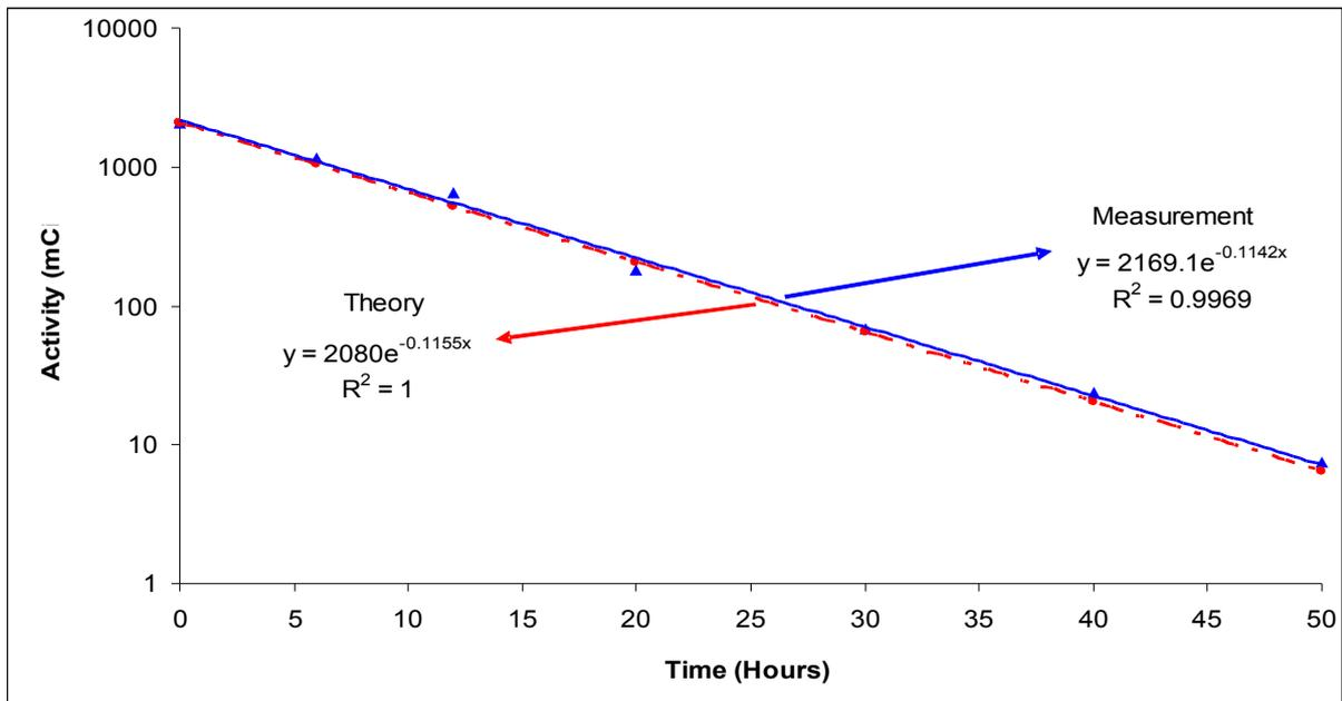
**Figure 8:** Linearity results using the decay method for CRC-15R dose calibrator.
