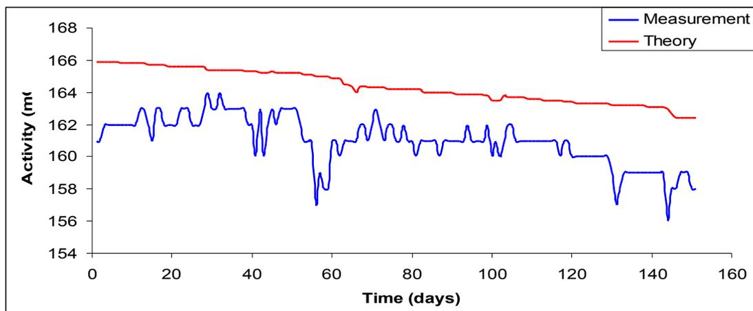
**Figure 2:** Source constancy test for CRC-15R dose calibrator, using the  $^{137}\text{Cs}$  source reference.
