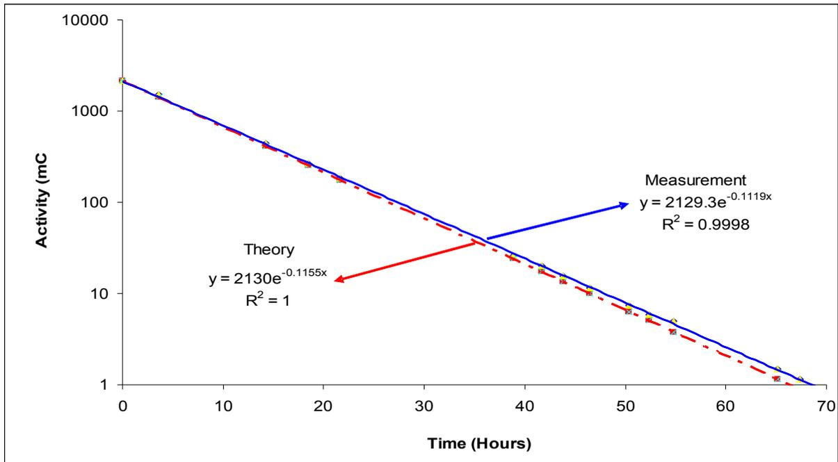
**Figure 7:** Linearity results using the Calicheck for CRC-15R dose calibrator.
