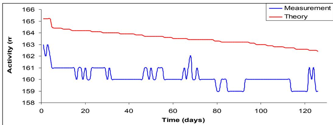
The reproducibility test results can be seen in figures 3 and 4. Both figures also are showing the upper and lower limits of acceptability, in our case this limits are at  $\pm 5\%$ . Here we do not perform any decay correction because the source reference used was the  $^{137}\text{Cs}$ , so there is not necessary this
