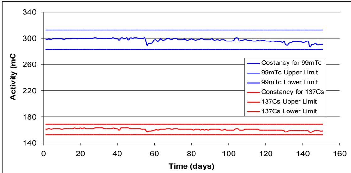
**Figure 4:** Reproducibility for CRC-15R dose calibrator, using the  $^{99\text{m}}\text{Tc}$  and  $^{137}\text{Cs}$  operating settings.
