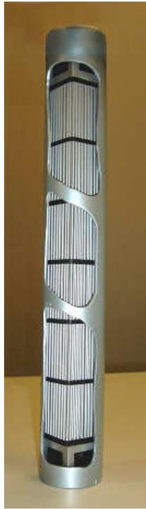
**Figure 6 – Preliminary Spent Fuel Canister**
