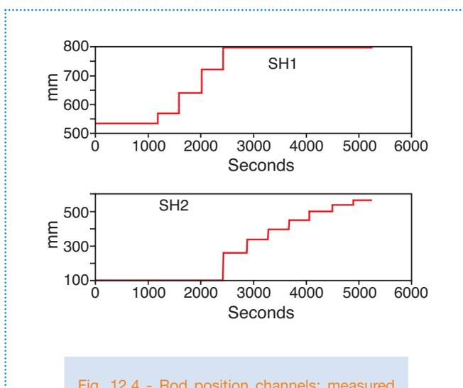
Fig. 12.4 - Rod position channels: measured data (blue); simulated data (red)
