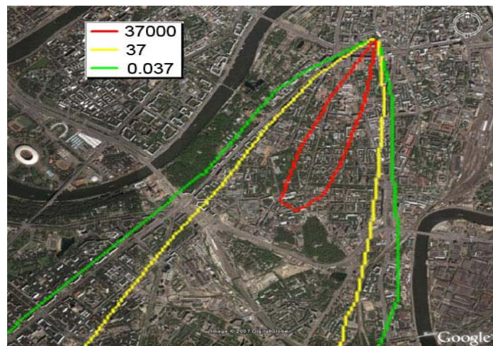
Figure 3. Forecasted density of urban territory contamination in case of blasting an explosive device stuffed with ^{137}\text{Cs} , \text{kBq/m}^2
