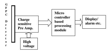
**Analog system:** It comprises of a charge sensitive preamplifier, followed by a discriminator and a mono stable multivibrator. The anode signal from each counter is fed to individual preamplifier-discriminator blocks, where they are first amplified and then converted in to TTL pulses. These pulses from individual counters are processed digitally in the microcontroller module.
