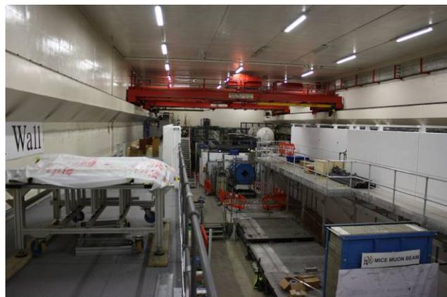
Figure 6: View of the MICE Hall, looking upstream. The wall separating the Hall from the ISIS vault is in the background of the photo, and the final quadrupole (blue) of the muon beam line is in the center. All of the remaining MICE components will be installed downstream of the quadrupole and upstream of the muon beam dump visible in the foreground.
