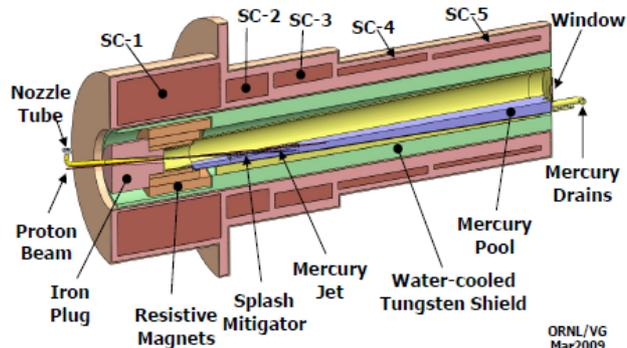
Figure 4: Hg-jet target concept studied in MERIT.
