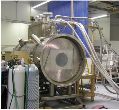
Figure 7: Spectrometer Solenoid being cooled down at Wang NMR. The first magnet will be delivered to RAL this summer.
