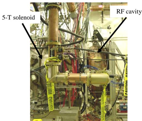
Figure 2: 201-MHz test cavity in the MTA.
