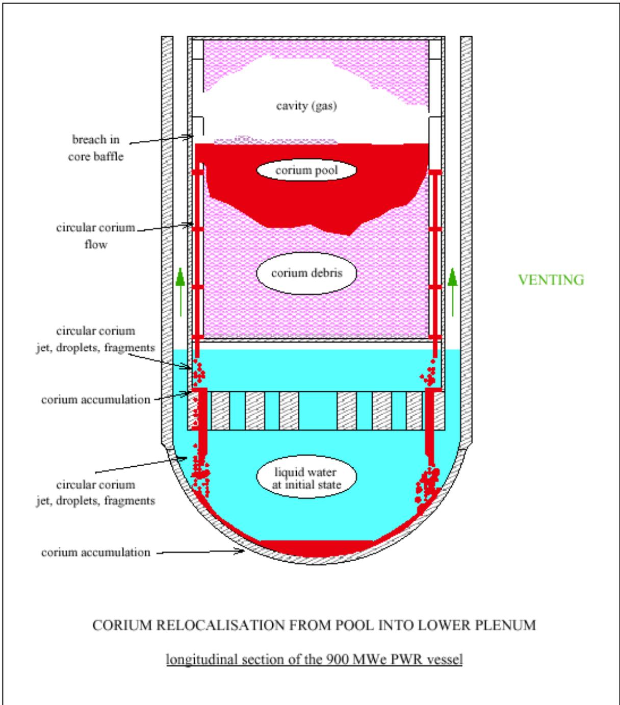
The simplified geometry of the 900 MWe PWR lower plenum vessels where the FCI takes place can be described with:
