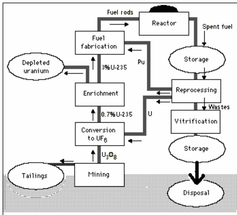
**Fig 1.** A generalized nuclear fuel cycle schematic
