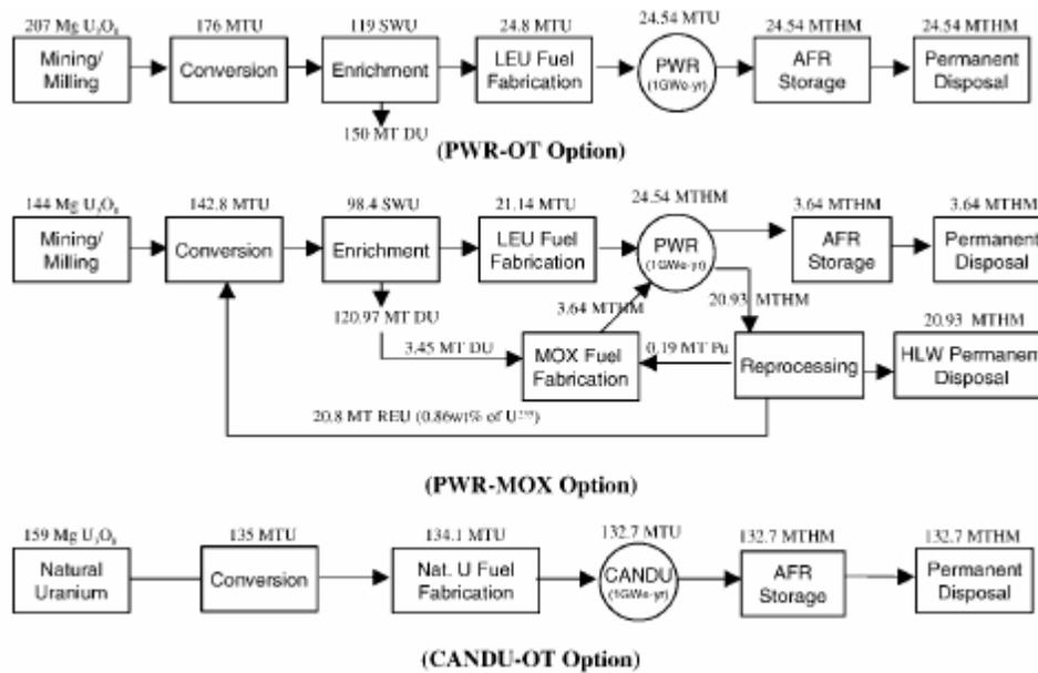
Fig (3): Material balance requirements for 1 GWe PWR and PHWR - NFC policies
