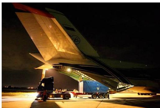
Fig 1. Loading spent fuel in ISO container into AN-124-100 cargo aircraft
