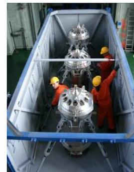
Fig 6. Loaded TUK-19 casks in ISO container
