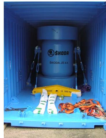
Fig.2. Arrangement of the SKODA VPVR/M cask in an ISO-container
