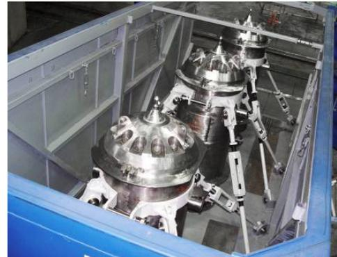
Fig.7. A freight ISO-container overpack for transportation of TUK-19 casks
