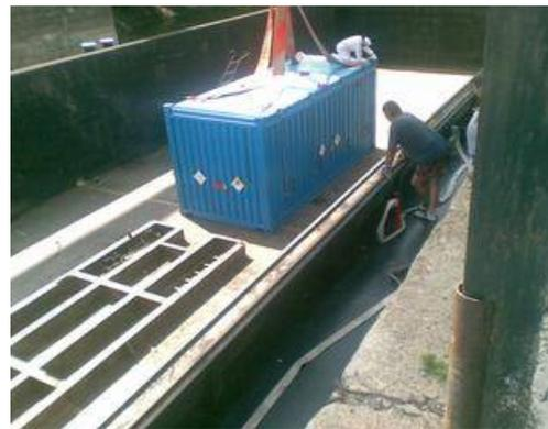
Fig.4. Loading of an ISO-container with SKODA VPVR/M casks on the river/sea barge
