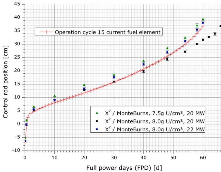
Fig 2: Predicted control rod driveway for different scenarios
