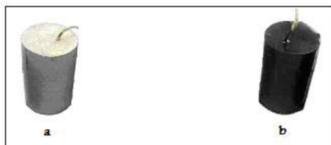
Fig. (1): Photo image of non-coated cement block (a) and that coated with bitumen emulsion (b)
