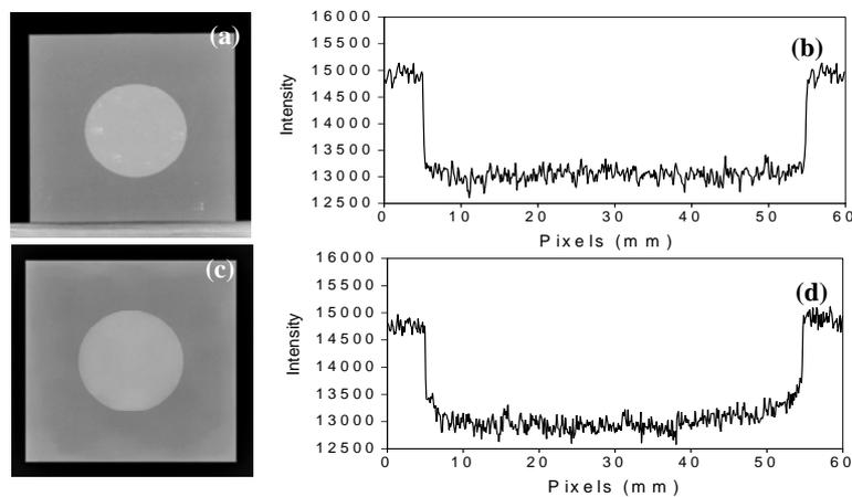
**Figure 11. 80 kV images of the test object. In (a), experimental image; (b) experimental image profile; (c) simulated image; (d) simulated image profile.**
