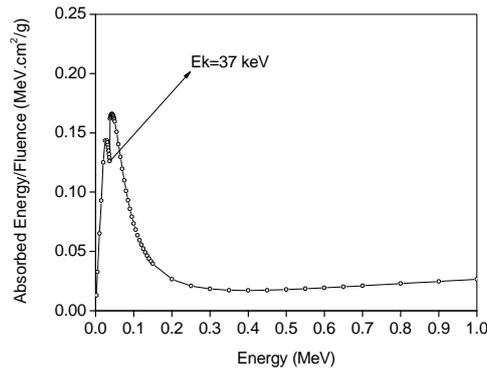
**Figure 1. Sensitive BaFBr material's response function. The values obtained were normalized by means of the fluence of photons emitted by the source.**
