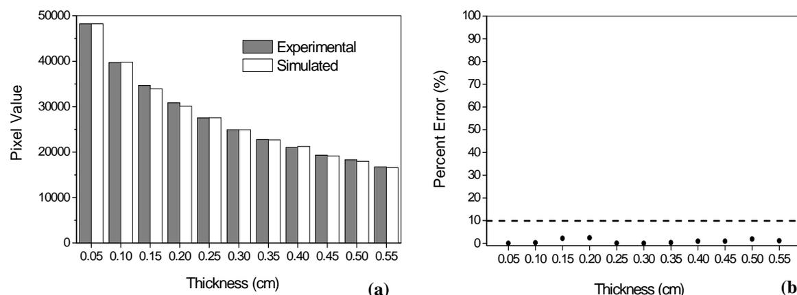
**Figure 7. A comparison between the pixel values obtained by means of the experimental images and the simulated images for the aluminum plates. In (a) pixel values and in (b) percent error.**
