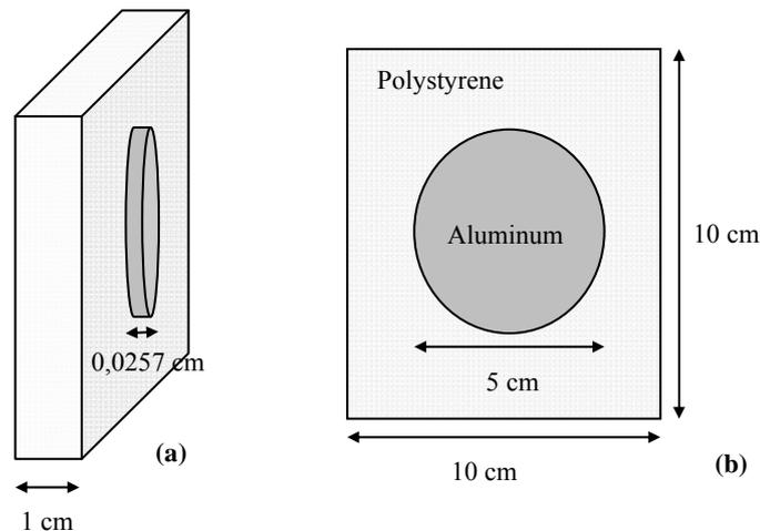
**Figure 9. Test object. In (a), a side view and in (b), a front view.**
