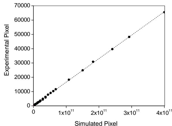
**Figure 2. The average arithmetical pixel values in the simulated detector based on the average arithmetical pixel values in the real detector. Data obtained for different values of air kerma incident on the detector.**
