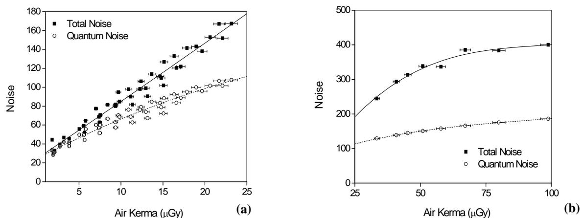
**Figure 3. Quantum noise and total noise based on air kerma incident on the BaFBr image detector. In (a), noises for the air kerma range from 1 to 25  $\mu\text{Gy}$ , and (b) noises for the air kerma range from 25 to 100  $\mu\text{Gy}$ . Data obtained by means of experimental images of an object with a homogeneous composition and constant thickness.**
