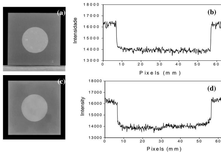
**Figure 10. 70 kV images of the test object. In (a), experimental image; (b) experimental image profile; (c) simulated image; (d) simulated image profile.**
