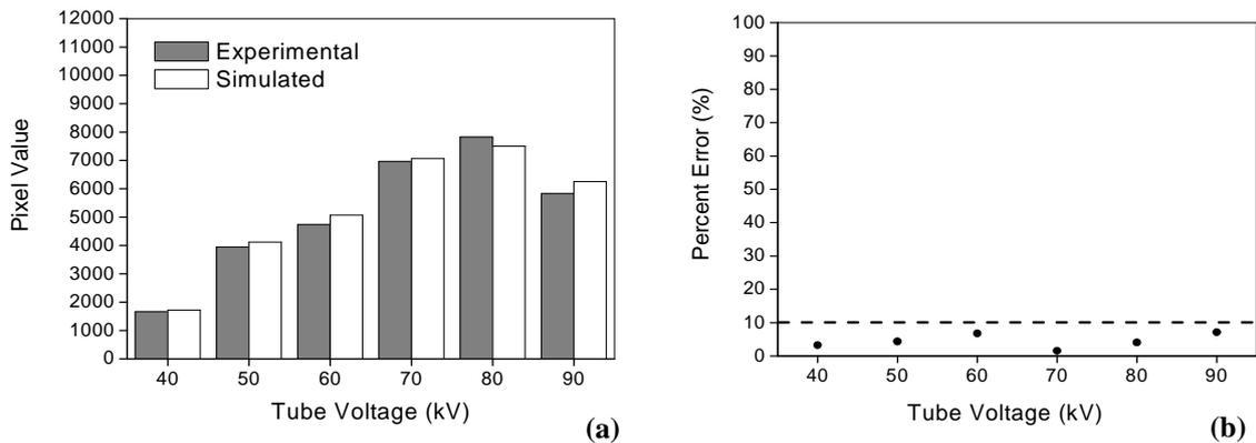
**Figure 8. A comparison between the pixel values obtained by means of the experimental images and the simulated images, varying the x-ray techniques employed. In (a) pixel values and in (b) percent error.**
