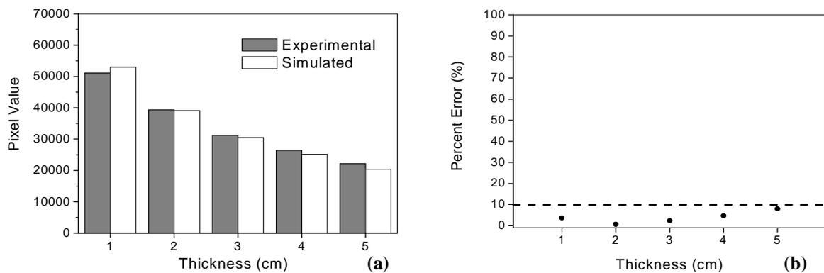
**Figure 6. A comparison between the pixel values obtained by means of the experimental images and the simulated images for the polystyrene plates. In (a) pixel values and in (b) percent error.**
