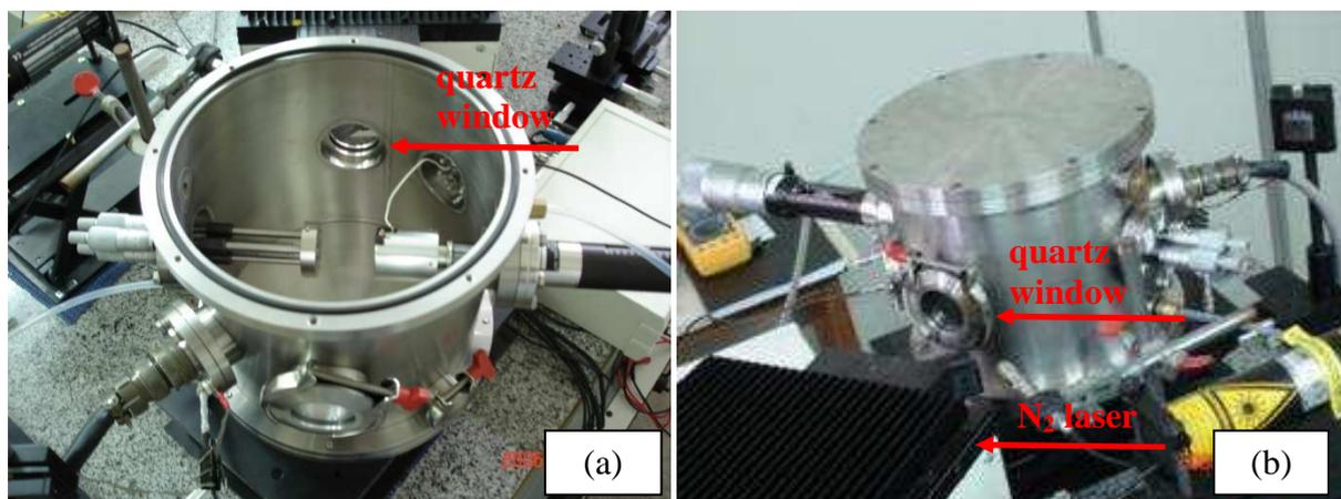
**Figure 1. (a) Electrodes inside the chamber (b) Laser-chamber configuration.**
