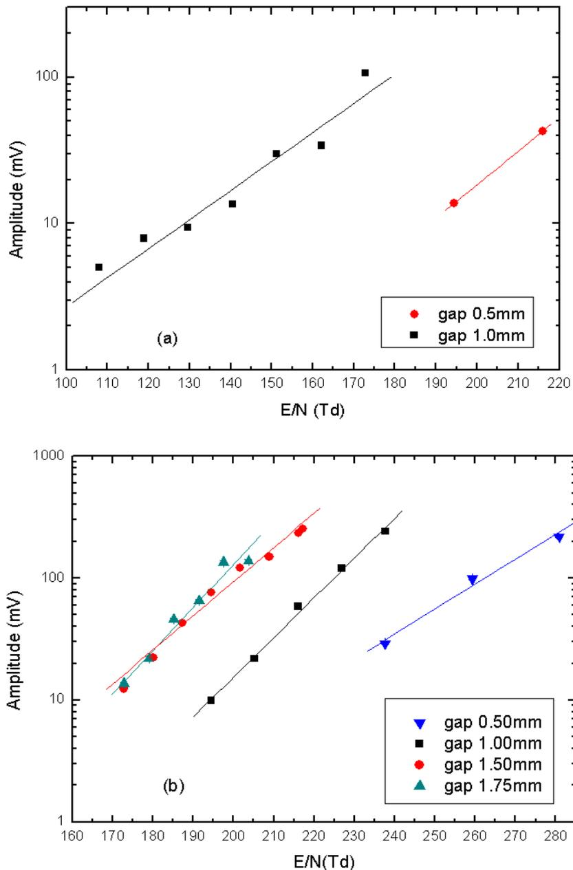
**Figure 3. Amplitude versus reduced electric field for (a) nitrogen and (b) isobutane.**
