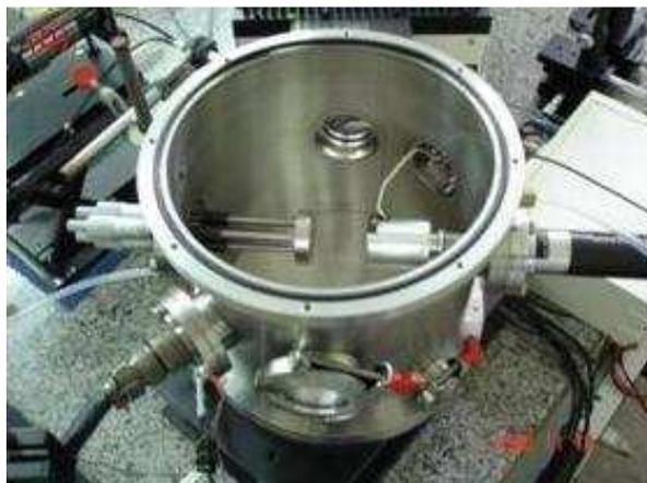
**Figure 1. The stainless steel chamber with the electrodes.**
