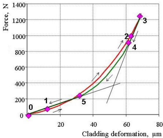
Fig.13. Typical diagram “force”- “deformation”
