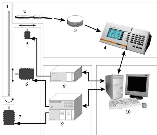
Fig.17. Equipment for oxide film thickness measurement: 1-fuel rod; 2-eddy-current probe; 3-signal amplifier; 4-signal processing unit; 5, 6, 7-stepper motors; 8, 9-stepper motor controller; 10-computer
