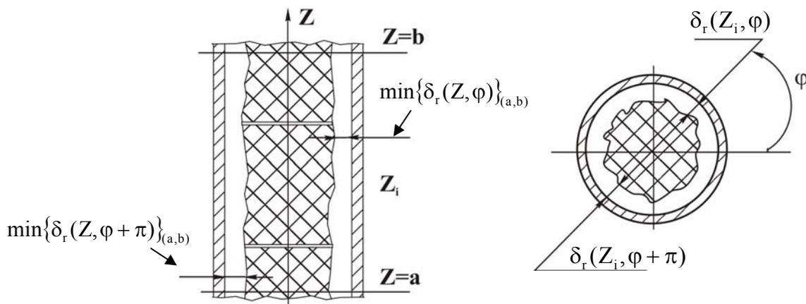
Fig.14. Schematic representation of the longitudinal section (a) and cross-section (b) of fuel rod
