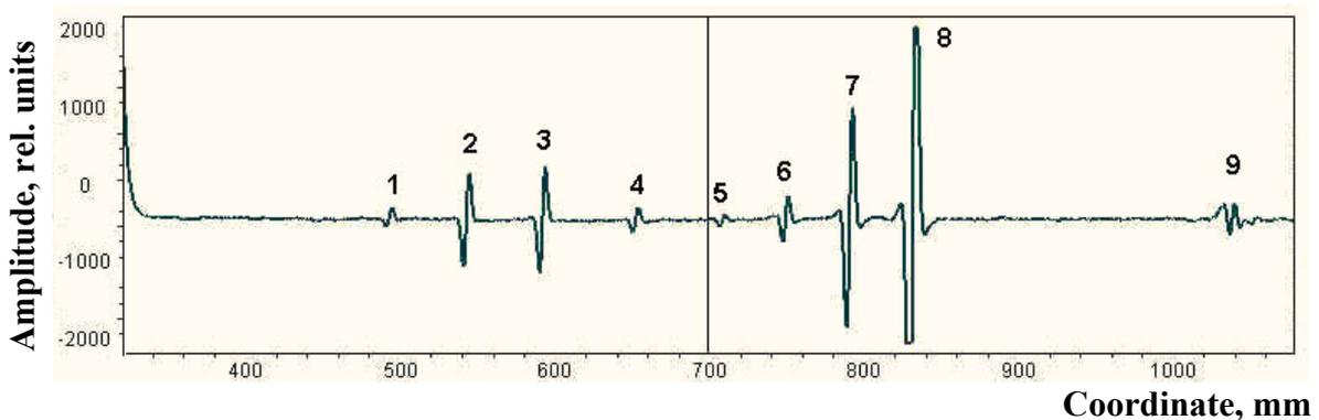
Fig.6. Diagram of the eddy-current probe signals from the artificially applied defects
