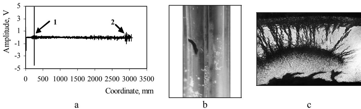
Fig.8. Results of eddy-current defectoscopy of the defect fuel rod: a-eddy-current diagram; b-appearance of the debris-defect; c-cladding microstructure in the region of the secondary defects; 1-signal of the debris-defect; 2-signals of the secondary internal defects.
