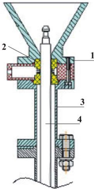
Fig.5. Positional of the eddy current probe and fuel rod under examination: 1-eddy current probe body; 2-measuring coil; 3-container for fuel rod; 4-fuel rod.
