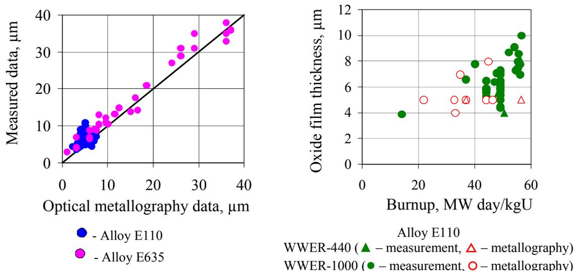
Fig.18. Results of method testing with the use of WWER fuel rods
