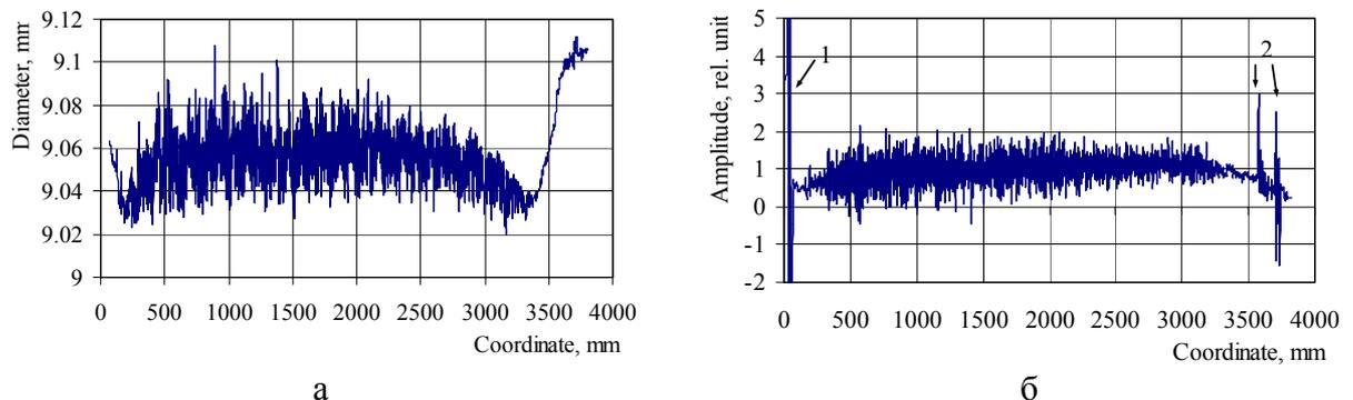
Fig.10. Results of diameter measurement (a) and defectoscopy by means of eddy-current method (b) of the WWER -1000 FR with a burnup of 55 MW·day/kgU: 1-signal of the plug; 2-signals of the fixing mechanism
