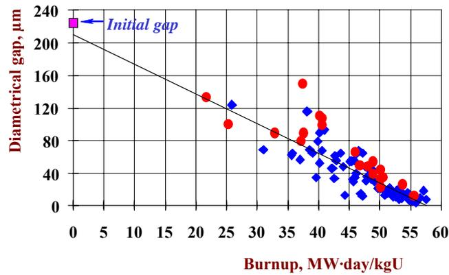
Fig.16. Diametrical fuel-cladding gap in the VVER-1000 fuel rods as a function of fuel burnup: ◆ - non-destructive testing; ● - optical metallography.
