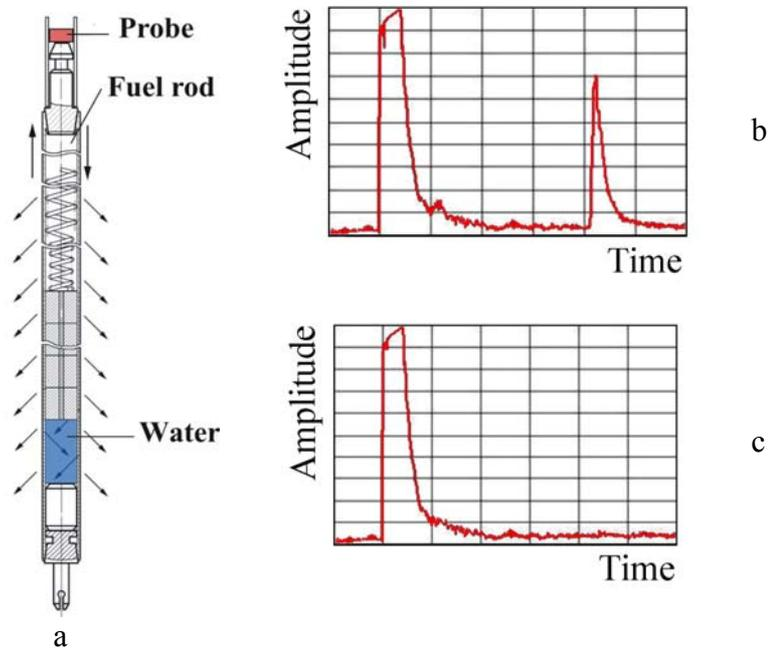
Fig. 1. Ultrasonic testing of failed fuel rods: 1 – schematic representation of fuel rod and fuel rod being tested; 2 – oscillogram of failed fuel rod; 3 – oscillogram of fight fuel rod.
