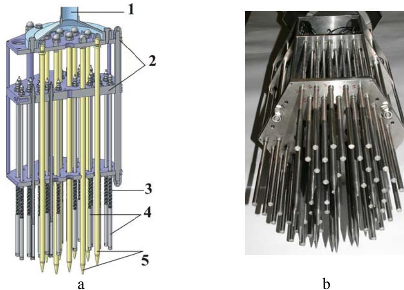
Fig.3. Sketch of the manipulator (a) and appearance of the lower part of the manipulator (b): 1-rod; 2-frame; 3-spring; 4-ultrasonic probes; 5-guiding pins.
