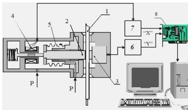
Fig.12. Scheme of diametrical gap measuring equipment: 1-fuel rod; 2-loading pin; 3-load sensor; 4-displacement transducer; 5-bellows; 6-charge amplifier; 7-amplifier; 8-analog-to-digital converter.
