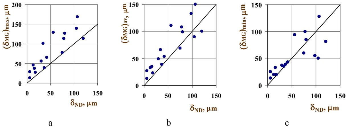
Fig. 15. Comparison between the non-destructive measurement results ( $\delta_{ND}$ ) and: a - maximum ( $\delta_{MG}$ ); b - average ( $\delta_{MG}$ ); c - minimum ( $\delta_{MG}$ ) values of gap determined for the FR metallographic sections
