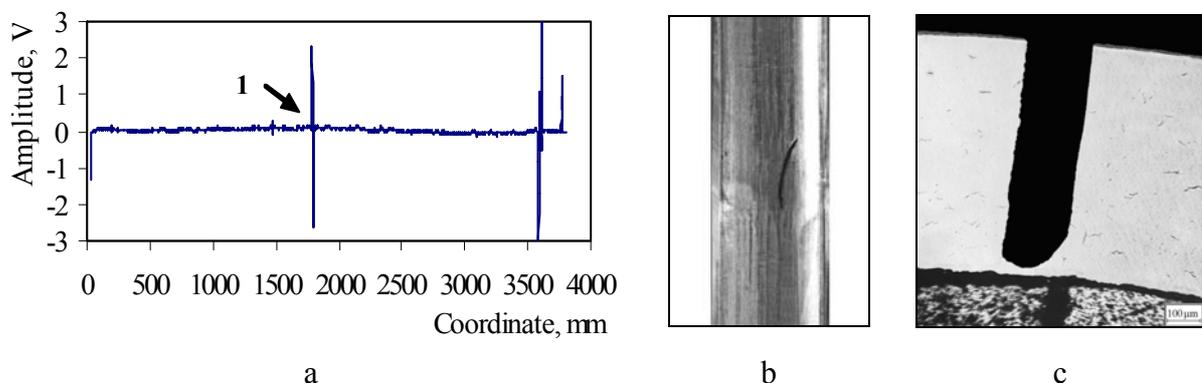
Fig.7. Results of the eddy-current defectoscopy of the FR cladding (a), outer appearance (b) and cross-section of the cladding with the part-through debris-defect: 1-signal of the debris-defect.
