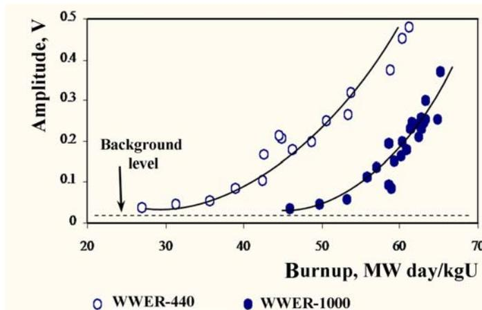
Fig.11. Magnitude of the eddy-current signal against fuel burnup
