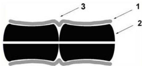
Fig.9. Formation of goffers: 1-cladding; 2- fuel pellet; 3-goffers.
