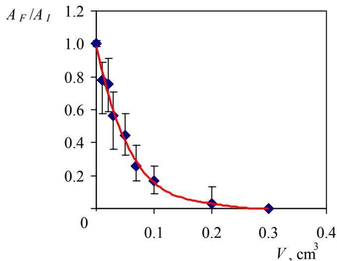
Fig. 2. Amplitude of the sensed signal against the water volume in the fuel –cladding gap of the dummy defect VVER FR
