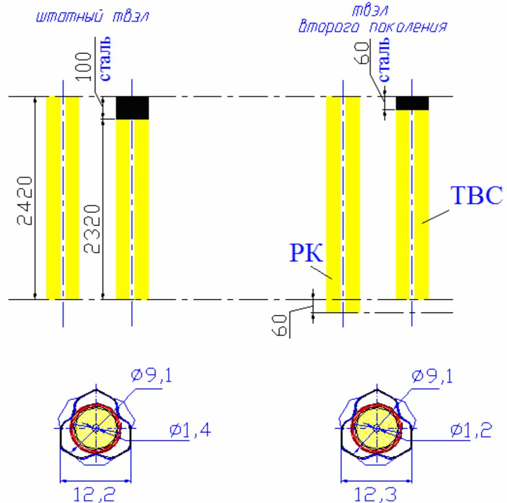
**Fig. 1 – Parameters of WWER-440 FA fuel pillar**
