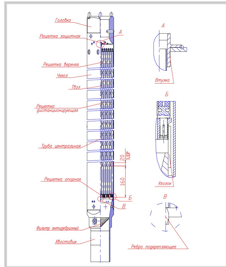
Fig. 2 – Second generation fuel assembly
