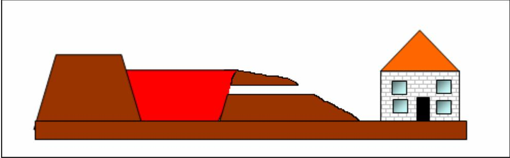
**Figure 4:** building of a house with full basement directly on the cover
