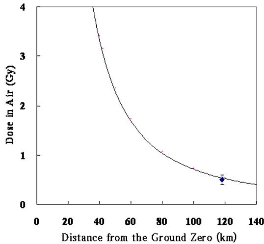
Fig. 2. Inspection of the RAPS calculation on degree of accuracy by a nuclear test case for a twenty kiloton surface nuclear explosion on August 29th 1949. The value of 47 kilometers per hour is applied for an effect wind velocity based on villager's testimony. ( ): the dose value in Dolon Village evaluated for a sample of brick by luminescence.
