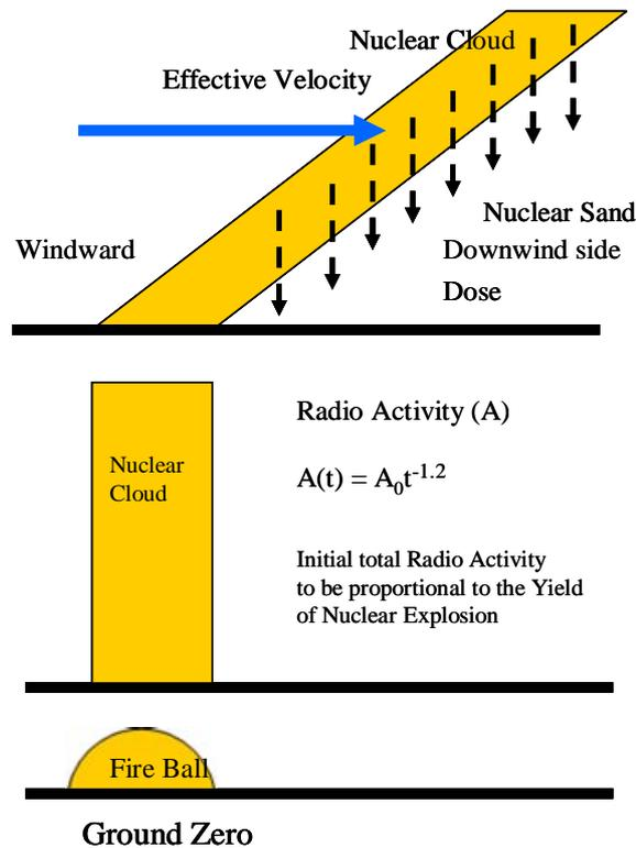
Fig.1 Chart of the dose calculation in a radioactive fallout zone by RAPS
