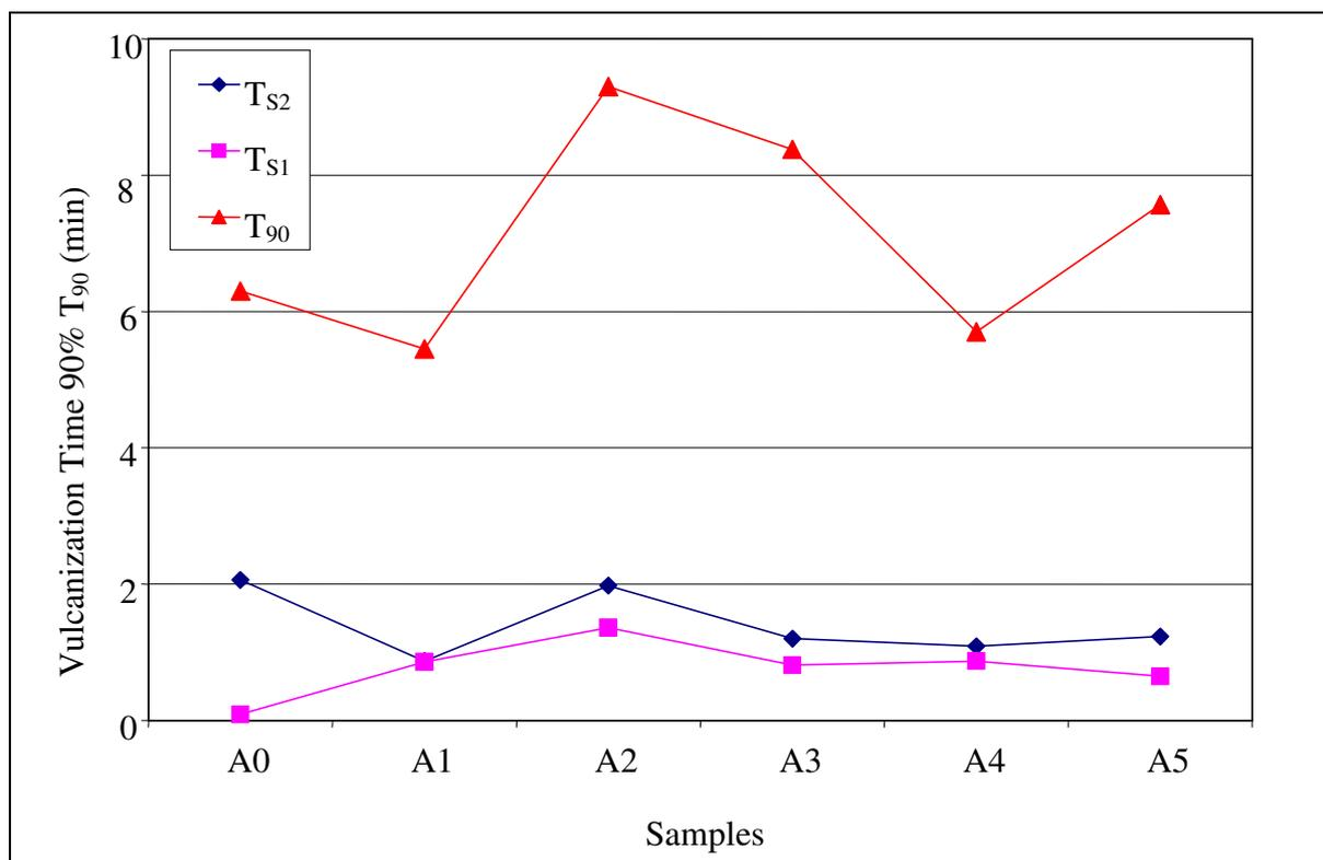
**Figure 4. Vulcanization parameters of vulcanized and devulcanized CR.**
