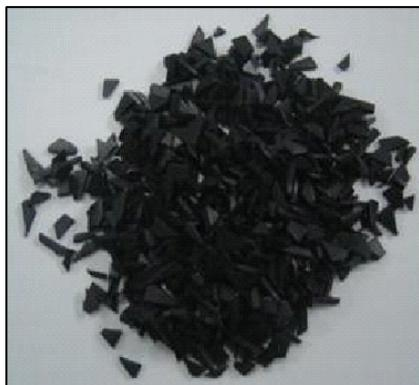
**Figure 2. Sample cut into small pieces from prepared sheet.**
