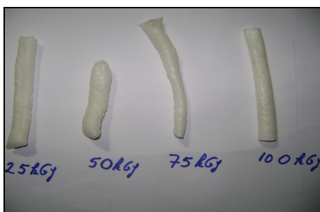
Figure 1. Appearance of gamma irradiated samples at 25, 50, 75 and 100 kGy.
