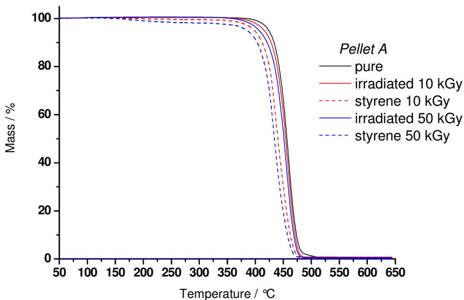
**Figure 2.** Thermogravimetric curves for pellets A pure, irradiated and grafted.
