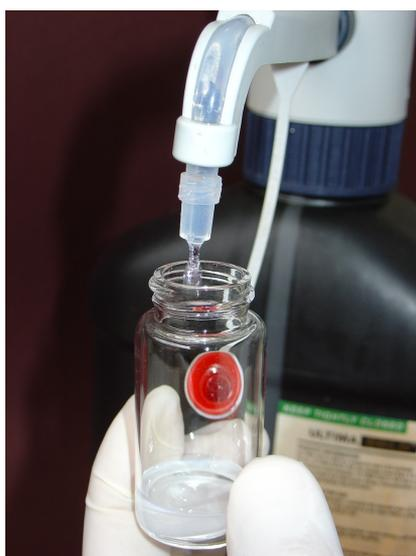
**Figure 2. Addition of LSC cocktail to glass vial containing a spiked water sample.**
