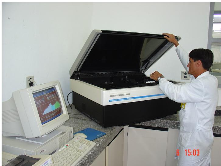
**Figure 1. Packard TRICARB 2700 Liquid Scintillation System**
