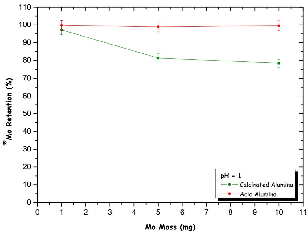
Figure 1- Curves of retention of Mo versus molybdenum mass (non-radioactive) by alumina columns at pH 1.
