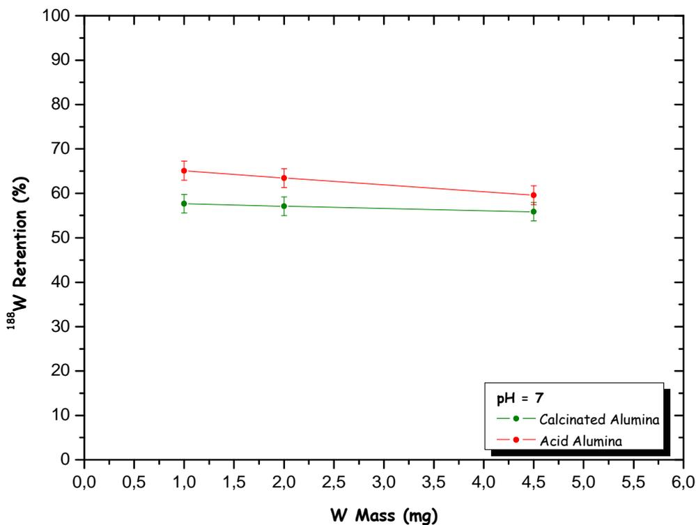
**Figure 3- Curves of retention of  $^{188}\text{W}$  versus tungsten mass (non-radioactive) by calcinated and acid alumina columns at pH 7.**
