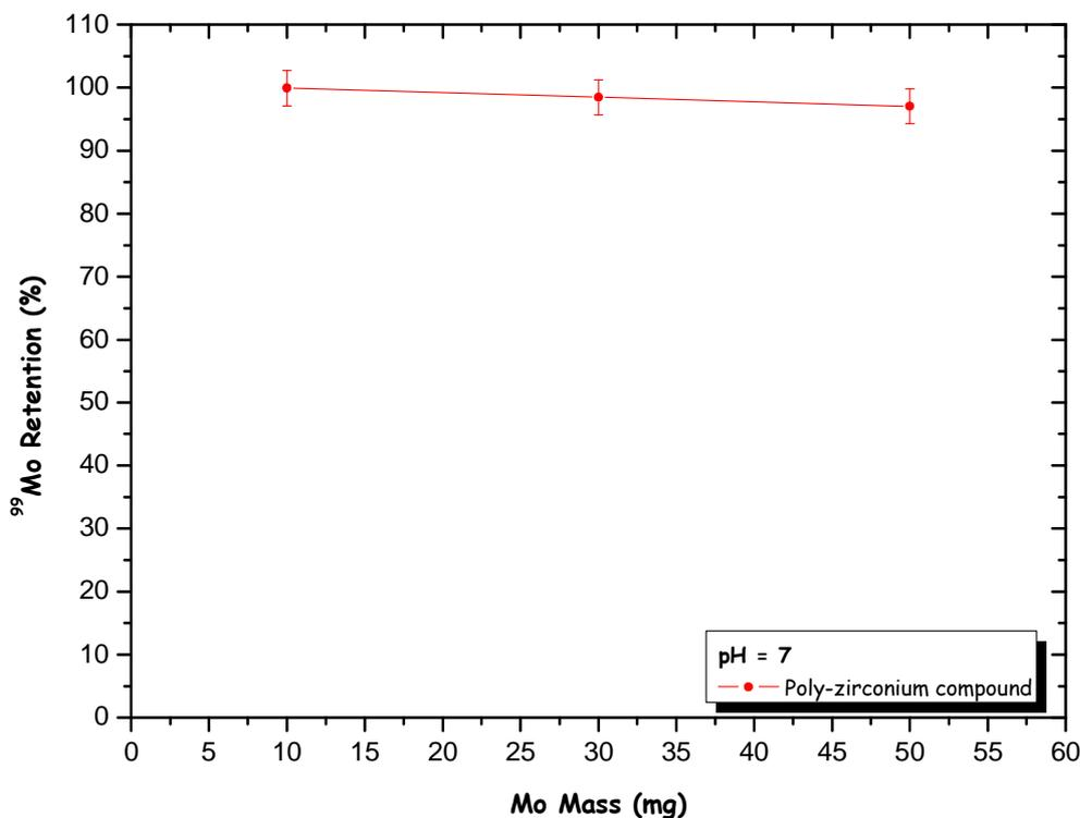
**Figure 2- Curve of retention of Mo versus molybdenum mass (non-radioactive) by PZC columns at pH 7.**
