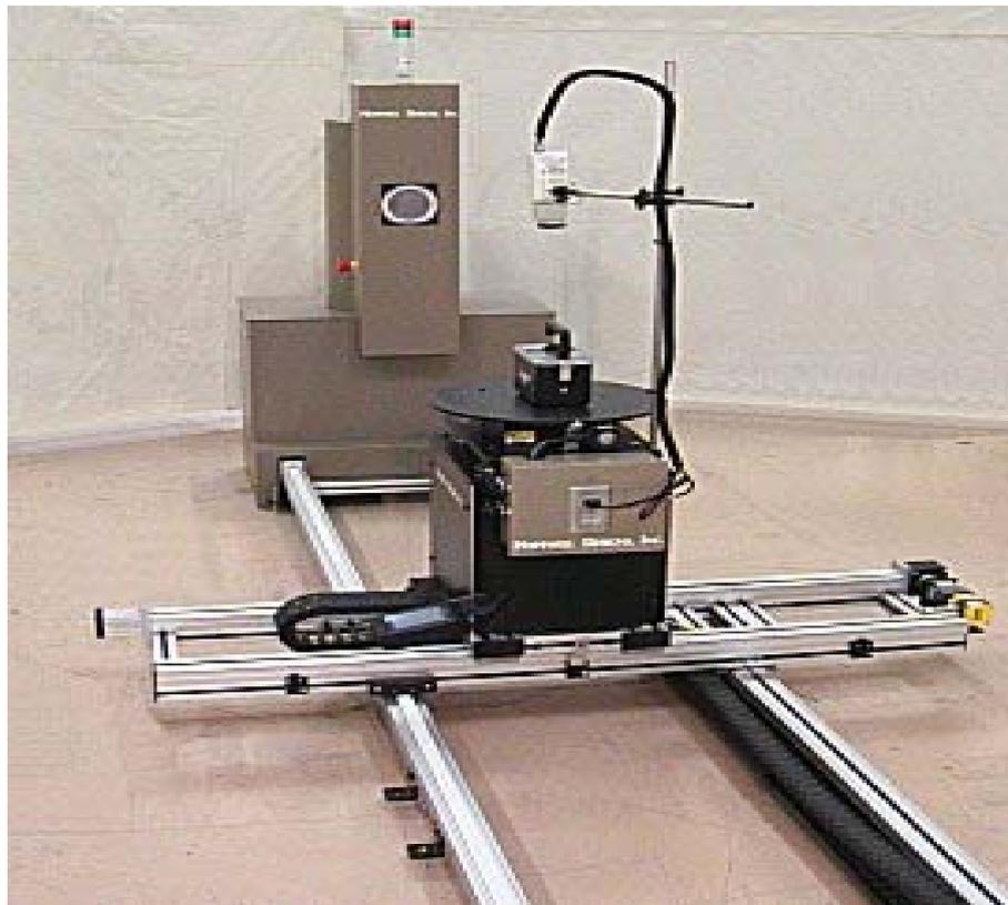
**Fig. 2. Linear positioning system, 2 axes.**
