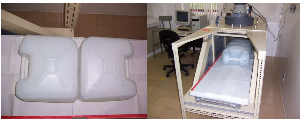
Figure 3. Phantom counting at CDTN-WBC system with bottles filled with standard solution
