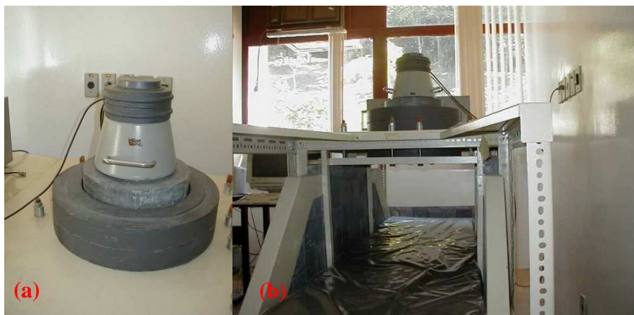
Figure 1. CDTN-WBC system: a) detector 6"x4" and b) geometry system
