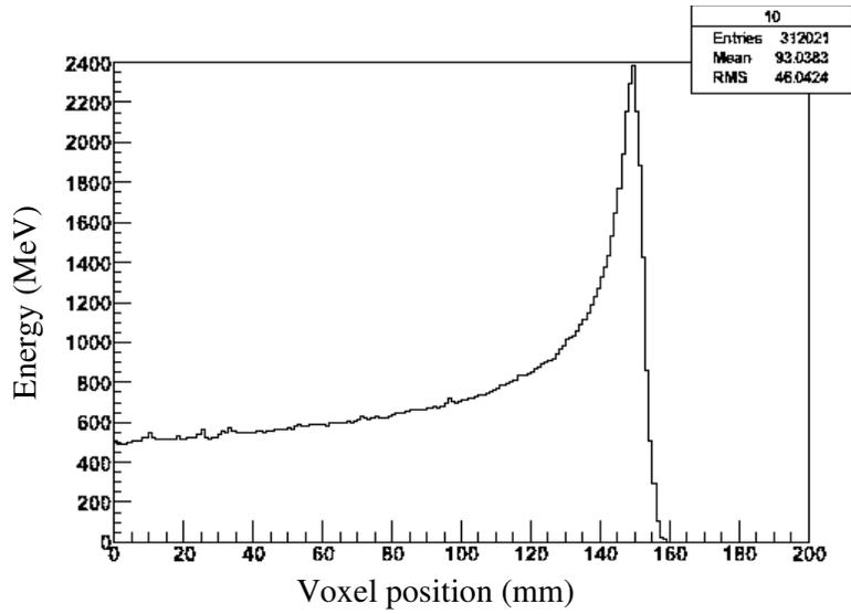
Figure 3: Deep profile of the energy deposited in a water phantom for a monoenergetic proton beam with average energy of 63.5 MeV.
