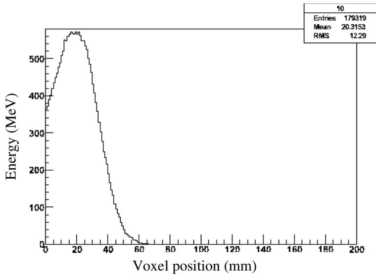
Figure 5: Deep profile of the energy deposited in a water phantom for a monoenergetic electron beam with average energy of 2 MeV.
