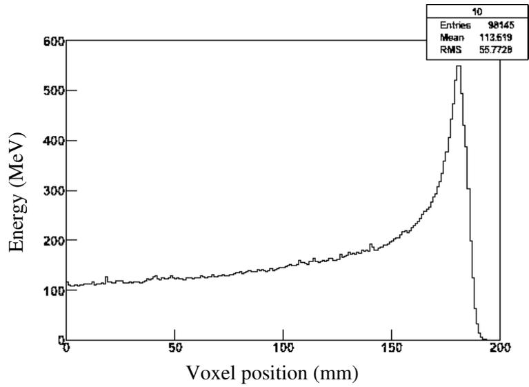
Figure 4: Deep profile of the energy deposited in a water phantom for a monoenergetic proton beam with average energy of 70 MeV.
