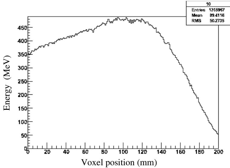
Figure 7: Deep profile of the energy deposited in a water phantom for a monoenergetic electron beam with average energy of 8 MeV.
