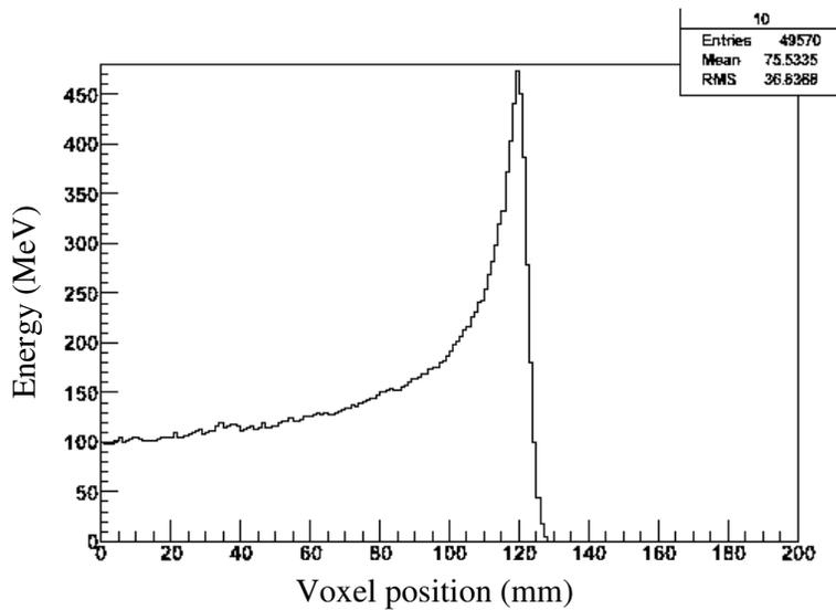
Figure 2: Deep profile of the energy deposited in a water phantom for a monoenergetic proton beam with average energy of 57 MeV.
