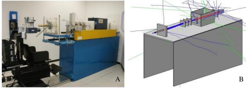
Figure 1: A) The real equipment for proton therapy, installed in Laboratorio Nazionale del Sud Institute of Physics nucleare in Nazionale di Catania, (B) simulated equipment used for the present simulation [6].
