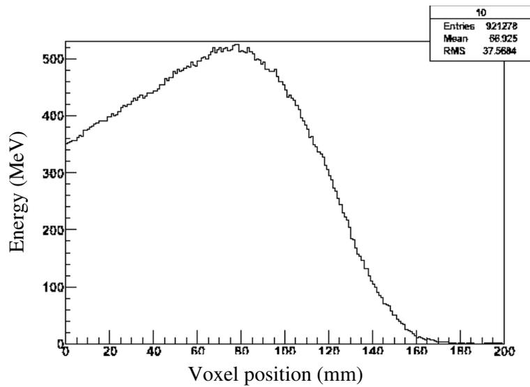
Figure 6: Deep profile of the energy deposited in a water phantom for a monoenergetic electron beam with average energy of 6 MeV.
