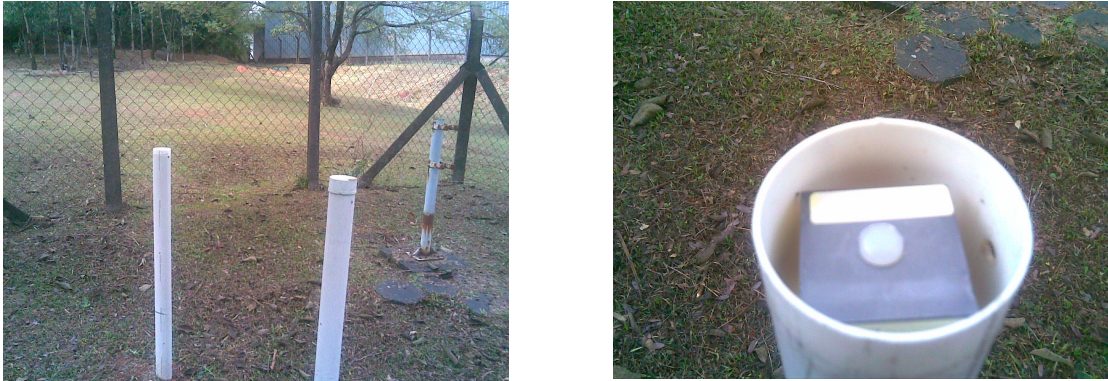
Figure 2: Place for the environmental monitoring. Left: the PVC rods. Right: DD positioned inside the rod.
