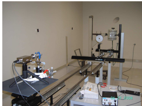
Figure 2. Experimental setup for x-ray spectrometry performed with the CdTe detector.
