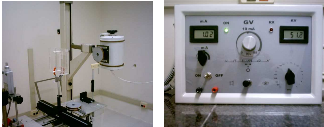
Figure 1. The single-phase x-ray unit with adjustable kV and mA. X-ray tube assembly (left) and control panel (right).
