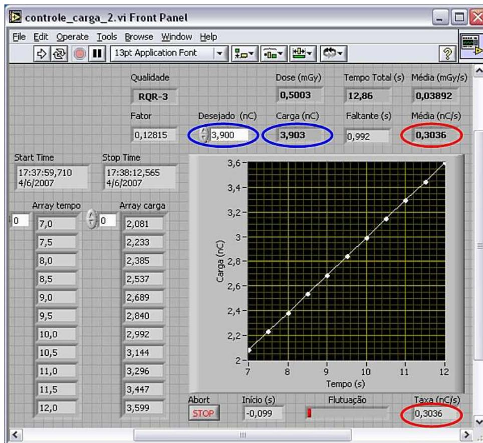
**Figure 1. Front panel of the charge control LabVIEW™ routine developed for test proofing the accuracy of the automatic shutter controller.**
