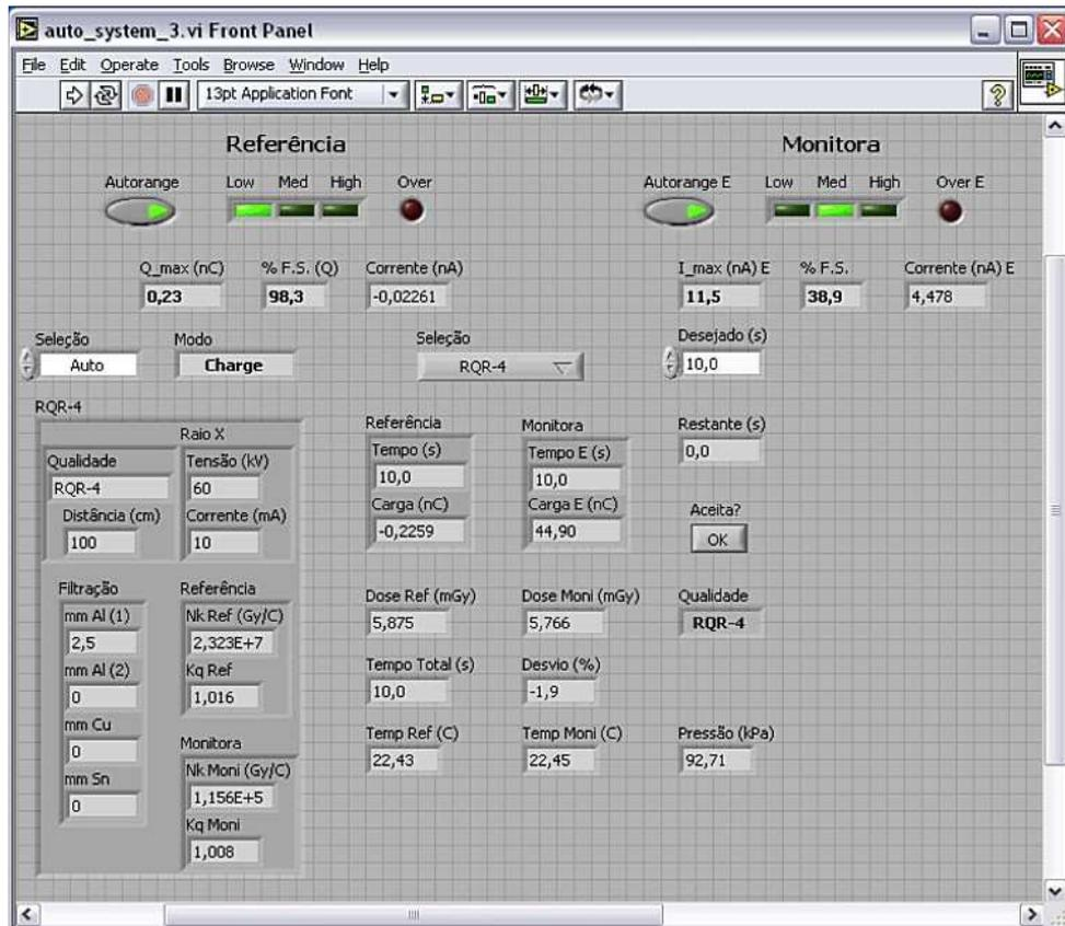
**Figure 2. Front panel of LabVIEW™ program developed for periodical generation of new calibration factors for the monitor chamber.**
