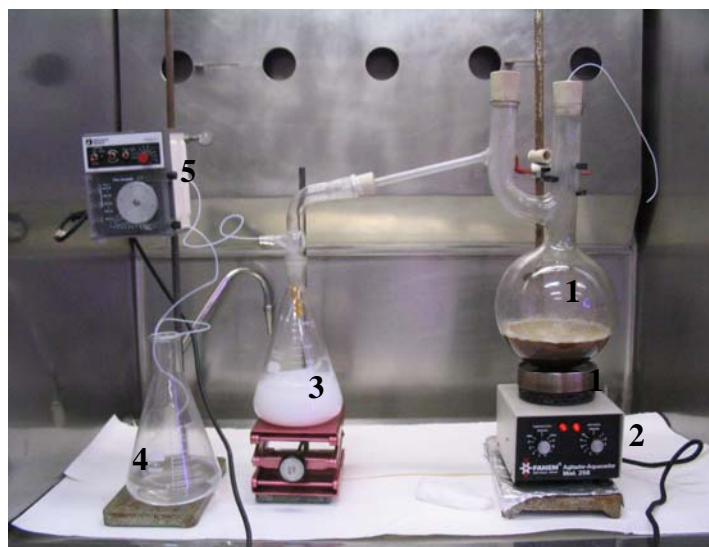
Figure 1. Experimental apparatus used in the degradation of the resin. 1. Resin + Fenton's reagent; 2. Magnetic stirrer; 3. Barium hydroxide solution; 4. Hydrogen peroxide solution; 5. Peristaltic pump.
