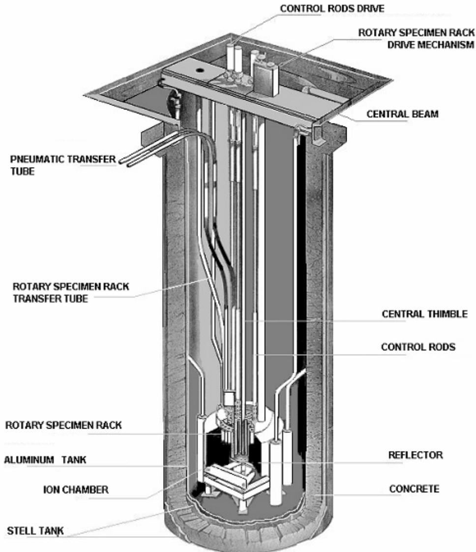
**Figure 2. Longitudinal section of the IPR-R1 TRIGA.**
