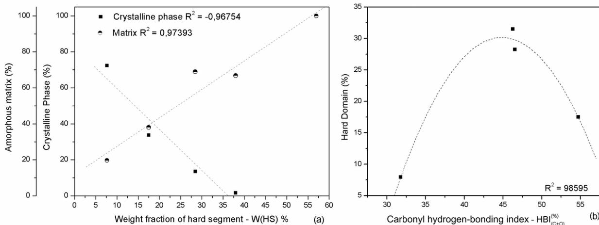
Figure 8 – Influence of hard segment content and  $HBI_{(C=O)}^{(\%)}$  on the multiphase structure of polyurethane.
