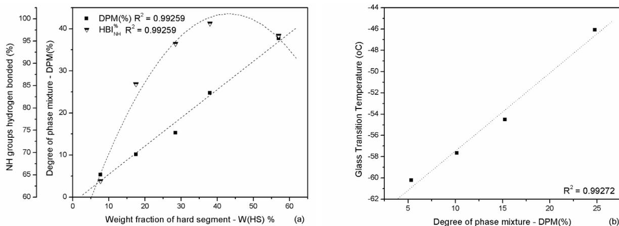
Figure 3 – (a) Influence of hard segment content on degree of phase mixture and (b) influence of the hard segment on glass transition
