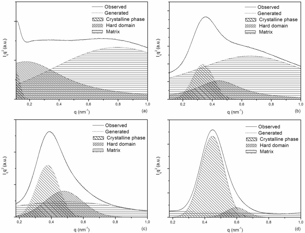
Figure 6 – Deconvoluted Lorentz SAXS patterns: (a)PU1250, (b)PU2000, (c)PU10000&530 and (d)PU10000.
