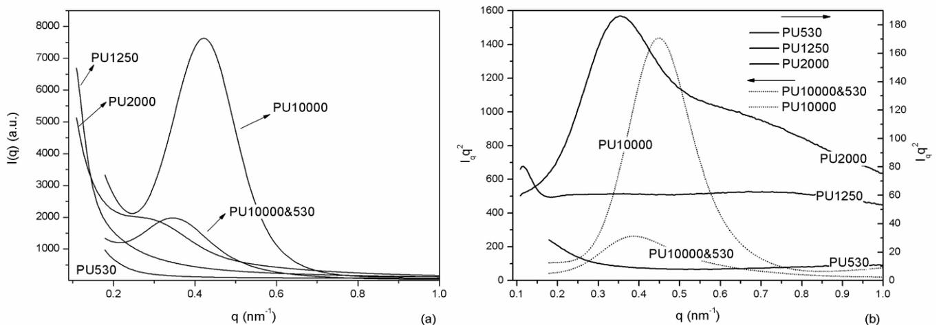
Figure 5 – (a) SAXS curves of obtained PUs and (b) Deconvoluted Lorentz SAXS pattern of samples
