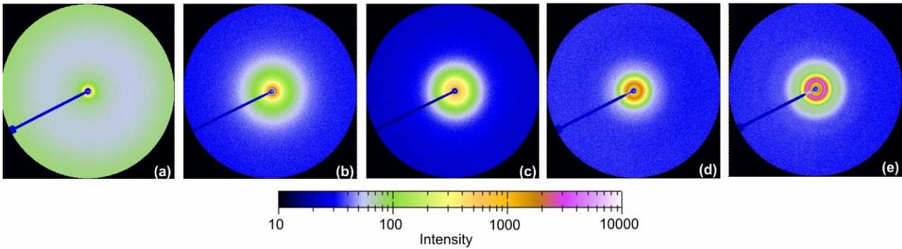
Figure 4 – SAXS pattern of: (a)PU530, (b)PU1250, (c)PU2000, (d)PU10000&530 and (e)PU10000.
