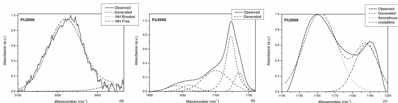
Figure 2 – Illustration of the deconvolution procedure used to determine the overlapped band of FTIR spectrum: (a) primary amine stretching, (b) carbonyl group stretching and (c) ether stretching.
