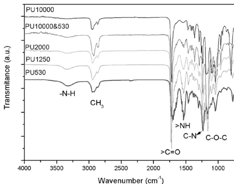
Figure 1 – FTIR spectra of PU530, PU1250, PU2000, PU10000&530 and PU10000 samples
