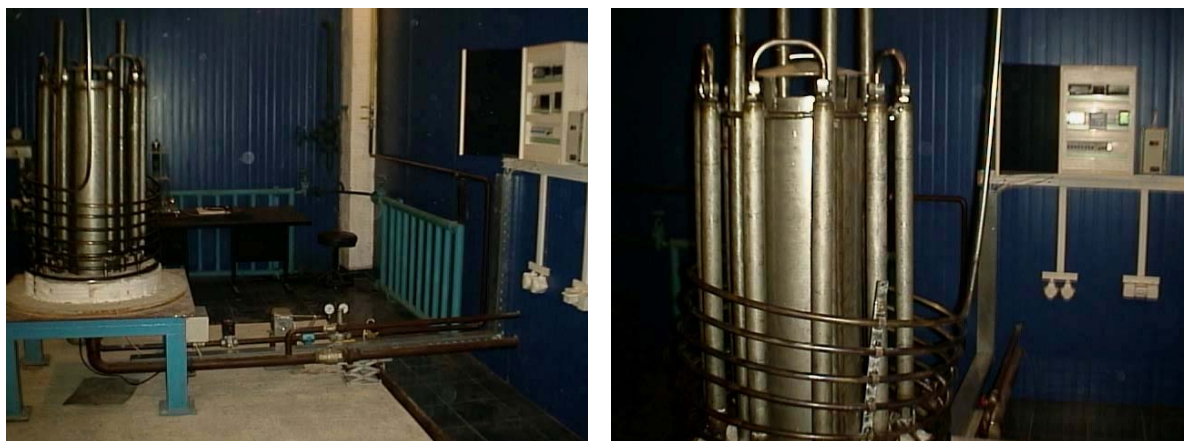
Fig. 1. Views from the reformer construction afferent to the experimental pilot for energy conversion using PEM fuel cells – „Blue Room”
