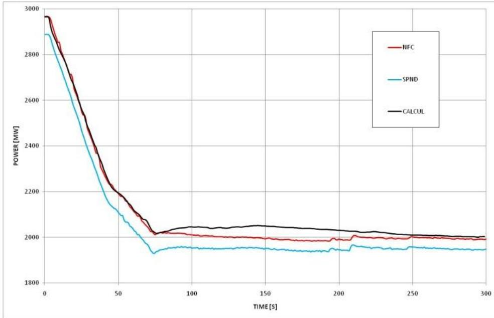
**Fig. 1** Comparison of calculated total reactor power evolution with measured by the FIC and SPND systems
