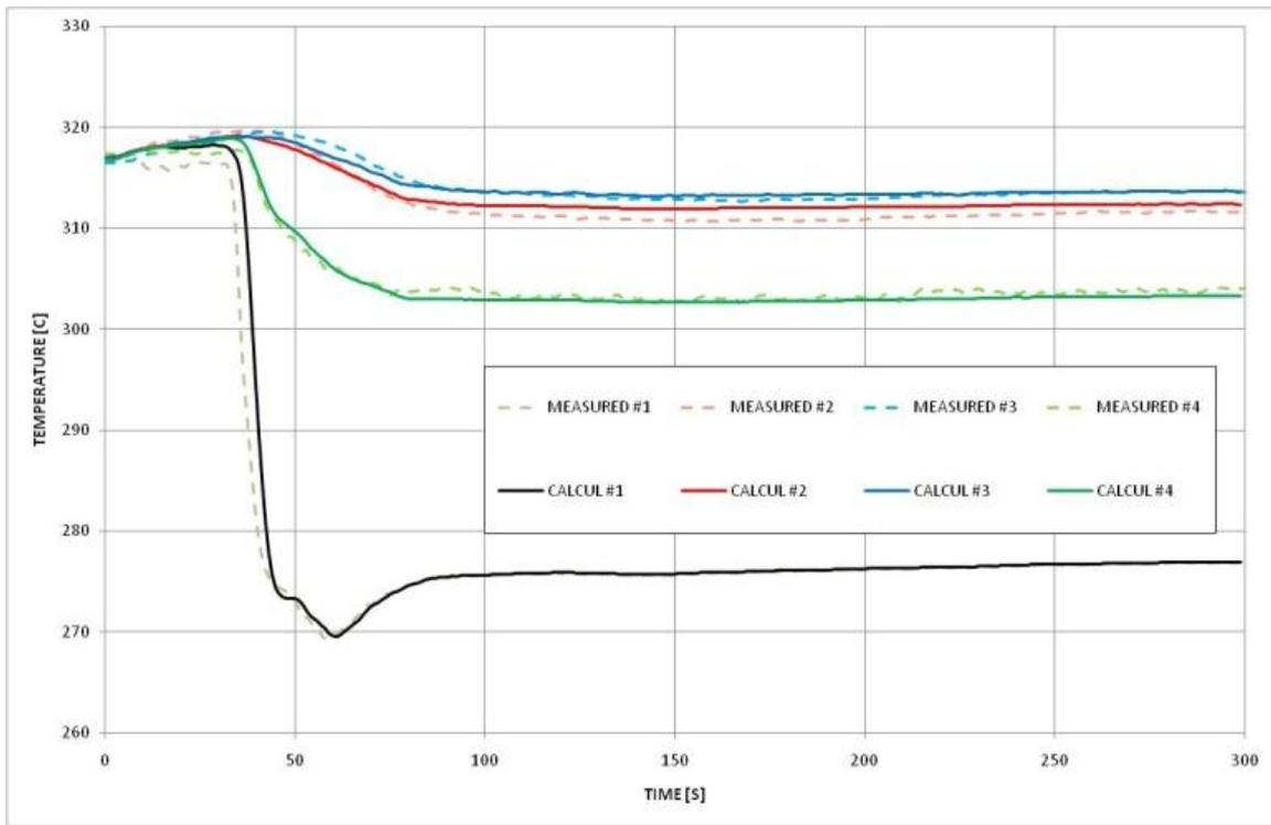
**Fig. 3** Comparison of predicted and measured hot legs' coolant temperatures
