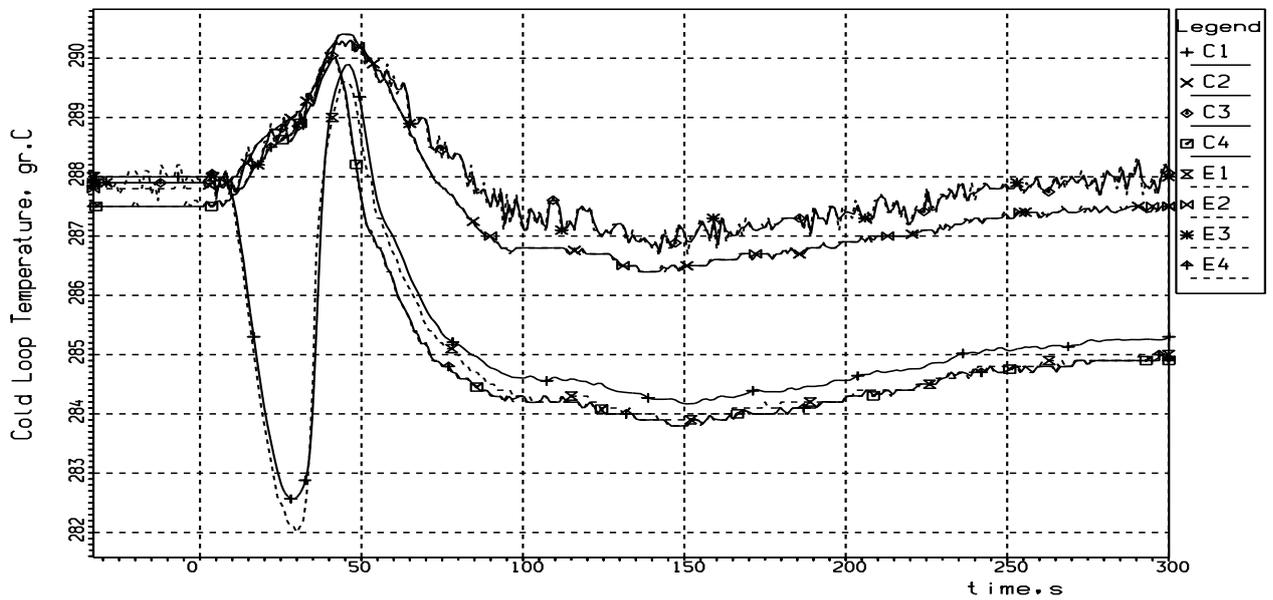
**Fig. 4** Comparison of predicted and measured cold legs' coolant temperatures
