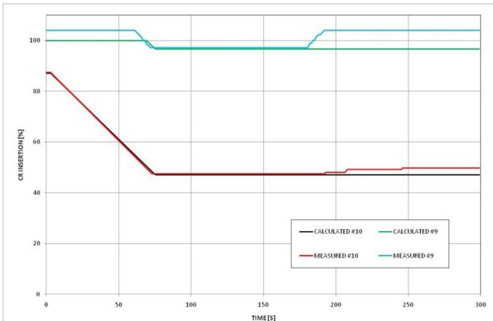
**Fig. 2** Comparison of predicted CRG #9 and CRG #10 insertion histories with the measured
