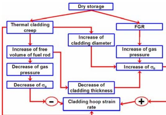
Fig. 14. The simplified flux diagram of the fuel rod behaviour under dry storage conditions (based on ref. 3).
