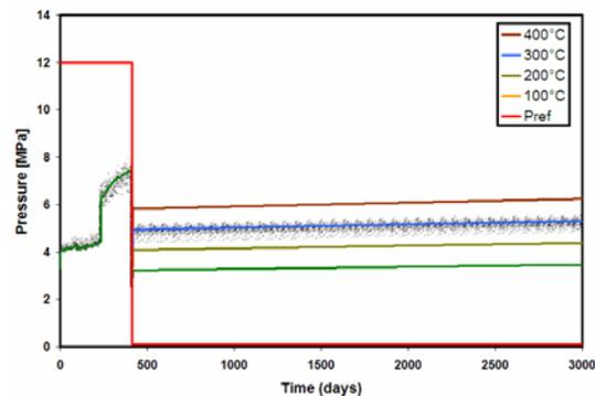
Fig. 21. The plot of the Fig. 17 including the statistical analysis of the inner pressure of the fuel rod due to the free gases in an Atucha I fuel rod for a storage temperature of 300°C.
