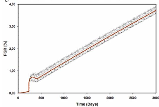
Fig. 20. The plot of the Fig. 16 including the statistical analysis of the fission gas release (FGR) of an Atucha I fuel during irradiation and dry storage (300°C of temperature for the storage device). The cloud of dots is a representation of the dispersion of the FGR calculations of BaCo.
