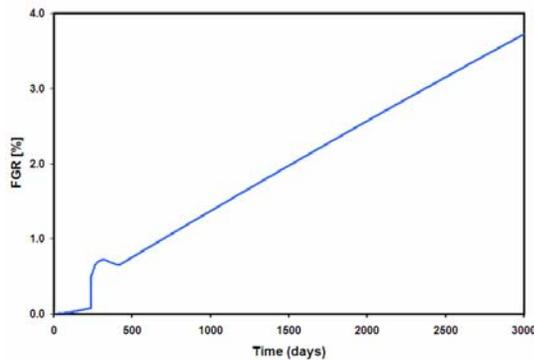
Fig. 16. The plot of the Fig. 15 but vs. time. FGR is due to a process thermally activated. Temperature of storage 300°C.
