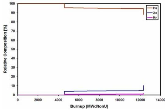
Fig. 7. Relative composition of the free gases in the empty places of the fuel rod (the Atucha I fuels is pre-pressurized)
