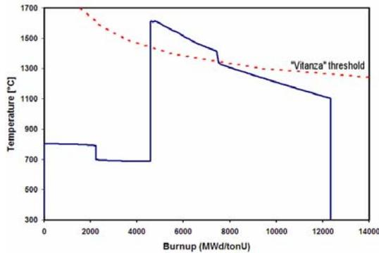
Fig. 2. Pellet centre temperature of the pellet in the 7th axial segment (the most demanding position) of a fuel rod of in the Atucha I NPP. The “Vitanza threshold” is included as a reference for the fission gas release.
