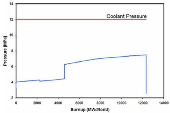
Fig. 11. Inner pressure of the fuel rod due to the free gases in an Atucha I fuel rod. The top curve is the coolant pressure of the Atucha I NPP. The fuel is under safe conditions ( $P_{coolant} > P_{gas}$ ).
