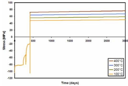
Fig. 18. Hoop stress (tangential stress) at the inner surface of the cladding at the 7th segment of an Atucha I fuel during the irradiation and the dry storage. The cladding is under a traction state at the dry storage conditions.
