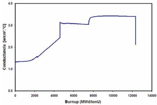
Fig. 10. Thermal conductance in gap pellet-cladding at the 7th segment of an Atucha I fuel.
