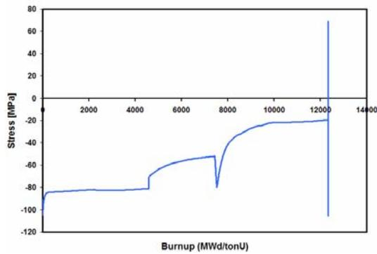
Fig. 13. Hoop stress (tangential stress) at the inner surface of the cladding at the 7th segment of an Atucha I fuel during the irradiation. The cladding is under a compression state up to the end of the irradiation.
