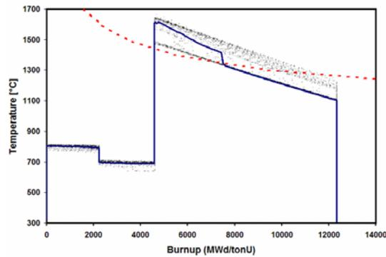
Fig. 19. Statistical analysis <sup>9</sup> of the fuel centre temperature at the 7<sup>th</sup> segment of an Atucha I during commercial irradiation. The cloud of dots is a representation of the dispersion of the thermal calculations of BaCo.
