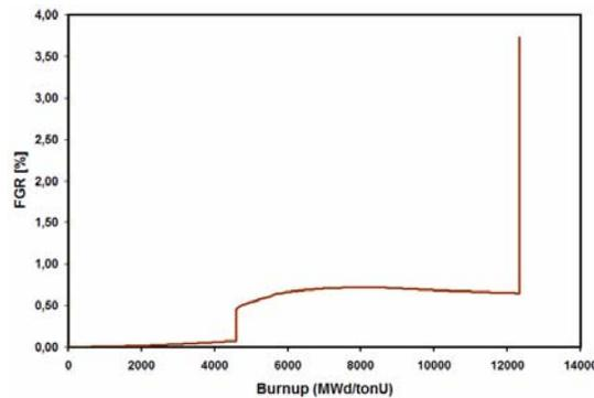
Fig. 15. Fission gas release (FGR) during irradiation and dry storage conditions for an Atucha I fuel in function of the average burnup. The FGR at EOL (“End Of Life”) is less than 1 %. The final peak is the release during dry storage at 300°C (without irradiation conditions –no burnup-).
