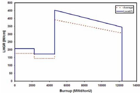
Fig. 1. A real and demanding power history of a SEU fuel of the Atucha I NPP. The dotted curve is the average linear heat generation rate (ALHGR) and the other one is the local LHGR at the 7th axial segment of the fuel.
