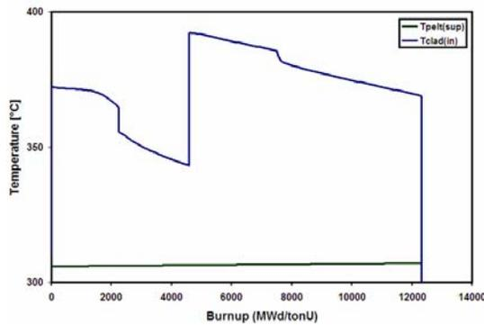
Fig. 3. Temperature in the gap between the pellet (top curve) and the cladding (lower curve).
