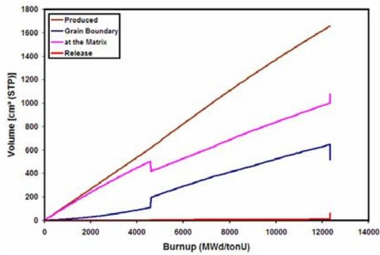
Fig. 6. Fission gases in the fuel rod. The top curve represents the fission gases produced during irradiation. The next curves are the fission gases in the matrix of the UO<sub>2</sub> grains and the gases at the grain boundary. The lower one is the fission gas released in the fuel rod.
