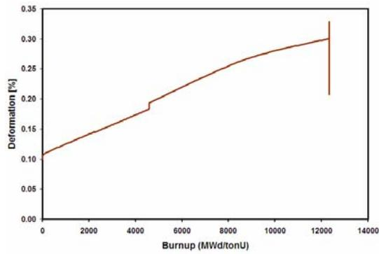
Fig. 9. Radial deformation of the cladding of an Atucha I fuel at the 7th axial segment.
