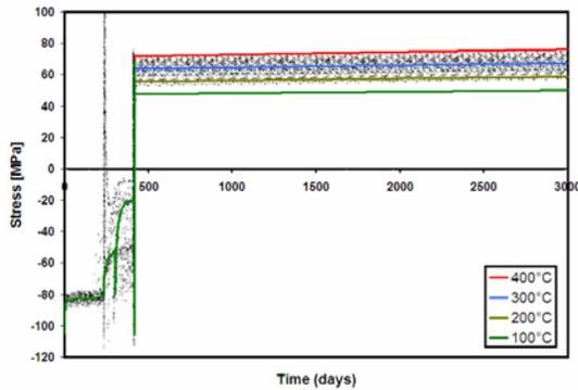
Fig. 22. The plot of the Fig. 18 including the statistical analysis of the hoop stress during the irradiation and the dry storage for an Atucha I fuel rod with a storage temperature of 300°C.
