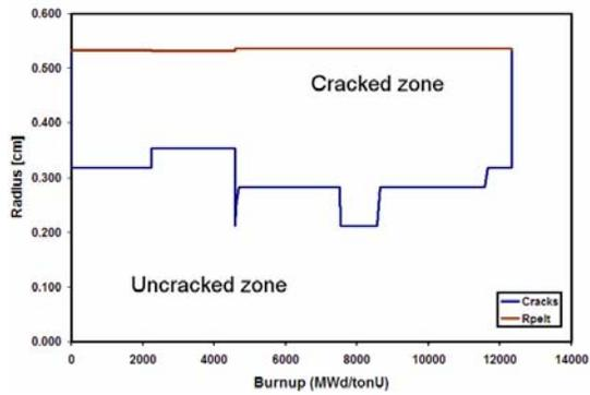
Fig. 12. Fuel pellet cracks opens due to tangential stresses at the most demanding axial position (7th from the top) of an Atucha I fuel. These cracks are not present in the centre of the pellet.
