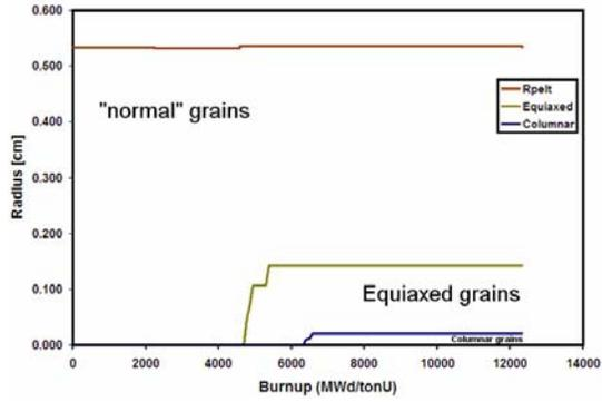
Fig. 4. Grain size evolution during irradiation at the 7th axial section of an Atucha I fuel. The top curve is the evolution of the pellet radius, the middle one is the limit for the equiaxed grains and the lower for the columnar grains. No central hole was found.
