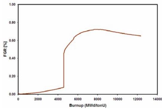
Fig. 5. FGR ("Fission Gas Release") in a fuel rod of the Atucha I NPP. The FGR at EOL is less than 1 %.
