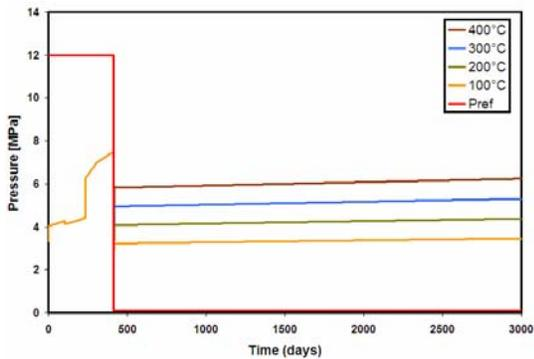
Fig. 17. Inner pressure of the fuel rod due to the free gases in Atucha I. The red curve is the pressure out of the cladding. We take into account four different temperatures for the storage.
