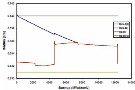
Fig. 8. Fuel rod radius evolution at the 7th segment of an Atucha I fuel during the irradiation. The parallel lines are the as fabricated pellet and inner clad radius. The top curve is the inner clad radius and the other one is the pellet radius. Pellet-clad contact is found over 6500 MWd/tonU.
