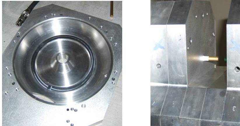
Figure 5.7: Tuning. View of the tuning ring after machining (left) and of the small tuner on the coupling cell (right)
