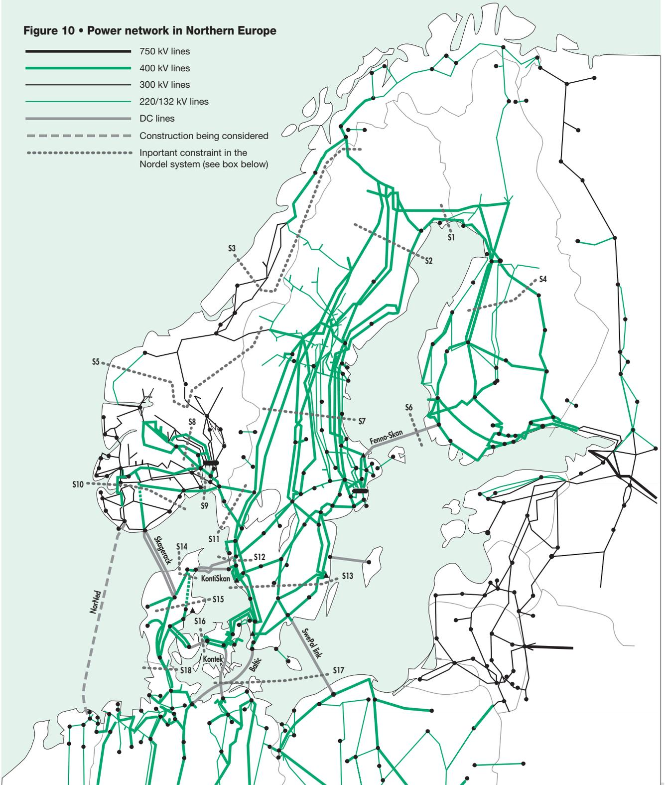
**Important constraints in the Nordel system (numbered from north to south)**
