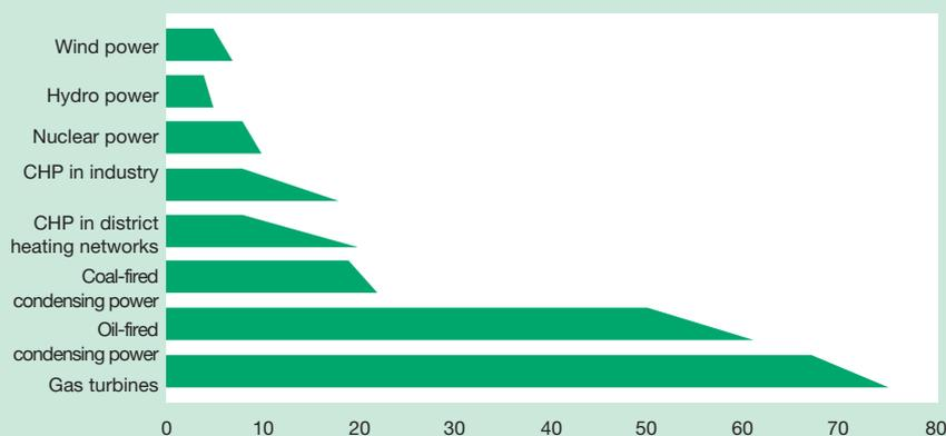
Figure 8 • Total electricity generation costs in new plants, öre/kWh
