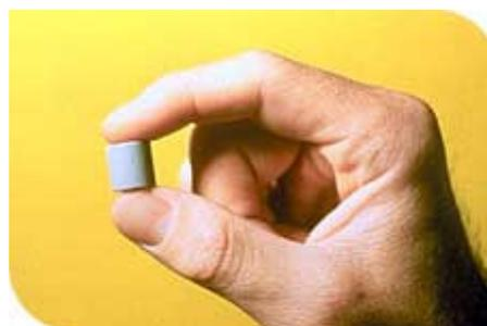
Figure 2. Uranium dioxide (UO<sub>2</sub>) pellet
