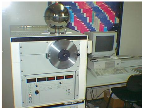
Figure 4. THQ Finnigan MAT mass spectrometer
