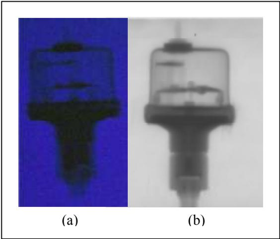
**Figure 7:** Some frames picked up from the actual footage of an ordinary lighter, placed upside down during the take, with an intentionally caused gas leakage. The darker vertical strips correspond to the liquefied gas.
