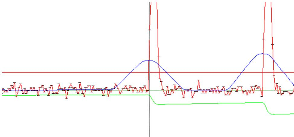
*Fig. 2: Signal (lower green curve); trigger filter (red, noisy line) and main filter (blue) values evaluated by MCA-527.*
