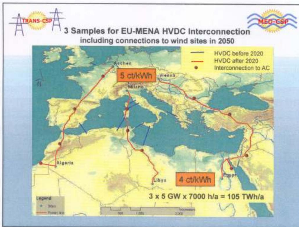
Fig. 11 Euro-MENA HVDC vs. AC interconnection schemes
