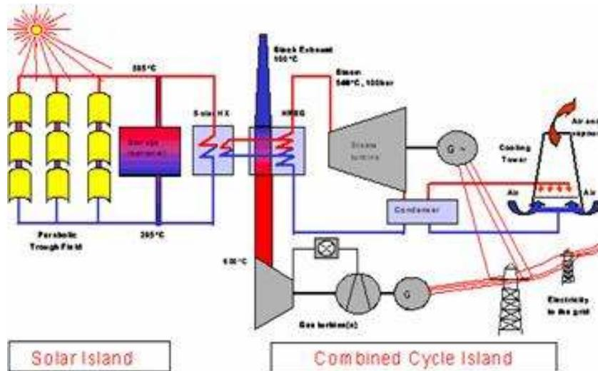
Fig. 8. Kuraymat Solar-thermal plant, schematic
