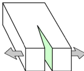
**Figure 7:** Mode I Fracture.
