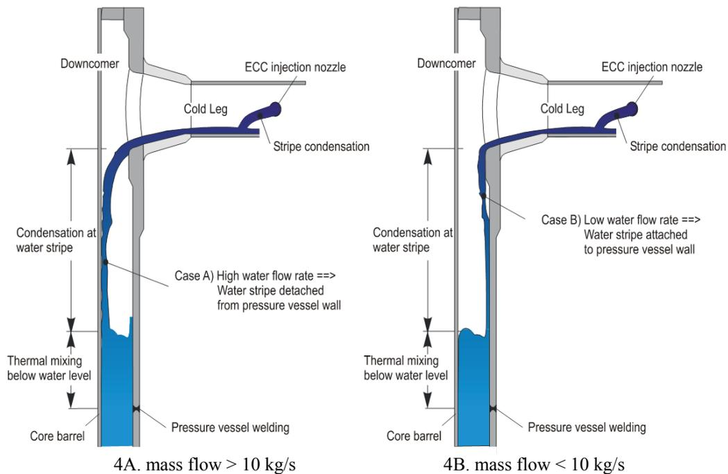
**Figure 4:** Safety Injection Flows into Voided Cold Leg (ref. E. F. Hicken, Thicket 2004).
