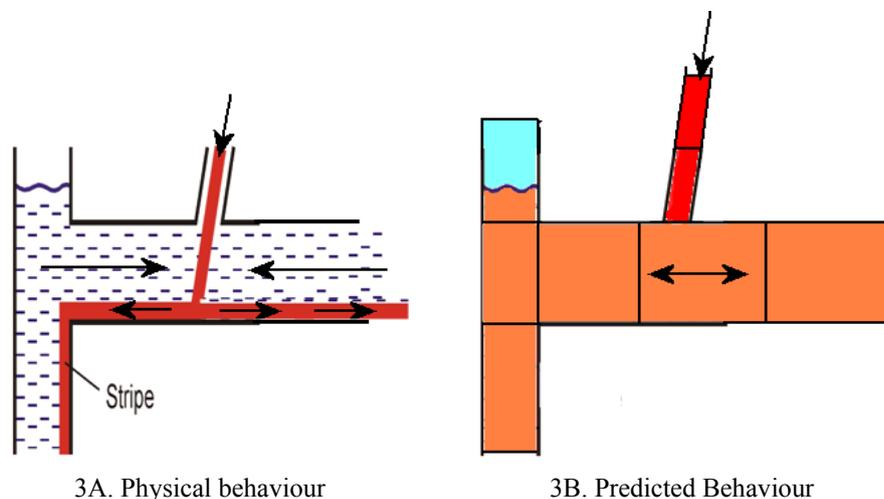
**Figure 3:** Behaviour of Fluid in Cold Leg during Safety Injection.
