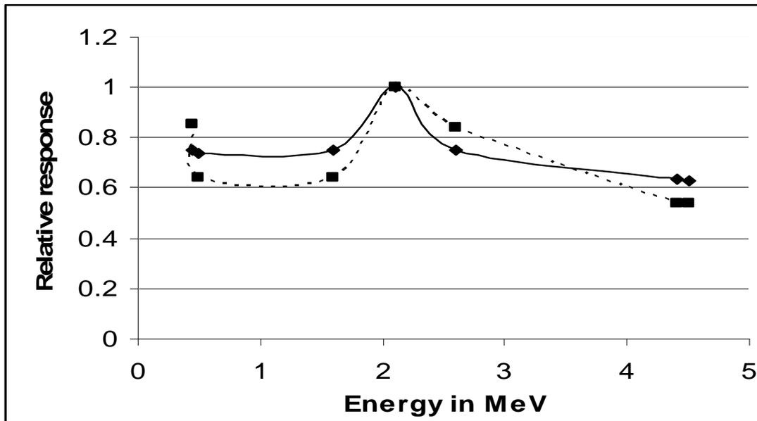
**Fig. 12:** Energy Response of CR-39 in ECE and CE Techniques normalized to  $^{252}\text{Cf}$  spectra. (Solid line -ECE technique ; Dotted line- CE technique)
