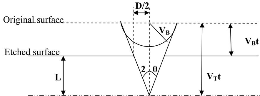
**Fig.2.** Track etch geometry for a normally incident particle (From Tommasino and Harrison, Radiation Protection Dosimetry,1985)
