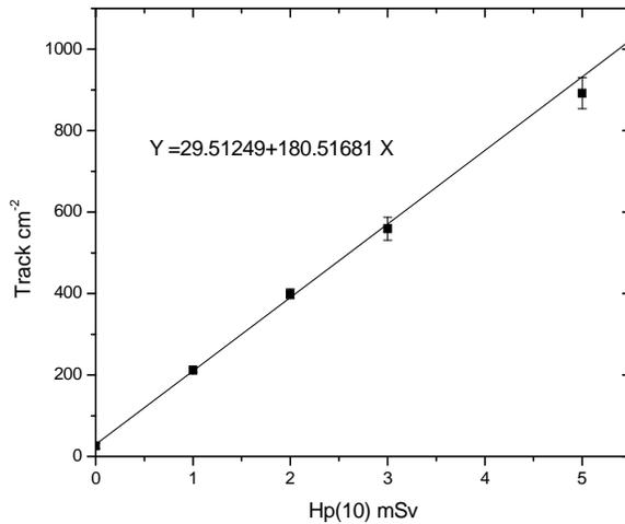
**Fig. 10:** Dose linearity of CR-39 using ECE technique in the dose equivalent range 1-5 mSv for <sup>241</sup>Am-Be fast neutrons. Calibration factor = 0.0058 mSv-cm<sup>2</sup> tracks<sup>-1</sup>
