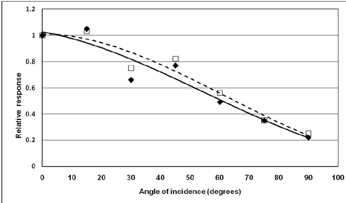
**Fig.13:** Relative response of  $H'(10,\alpha)/H^*(10)$  in free air (*dashed line*),  $Hp(10,\alpha)/Hp(10,0^\circ)$  on phantom (*solid line*).
