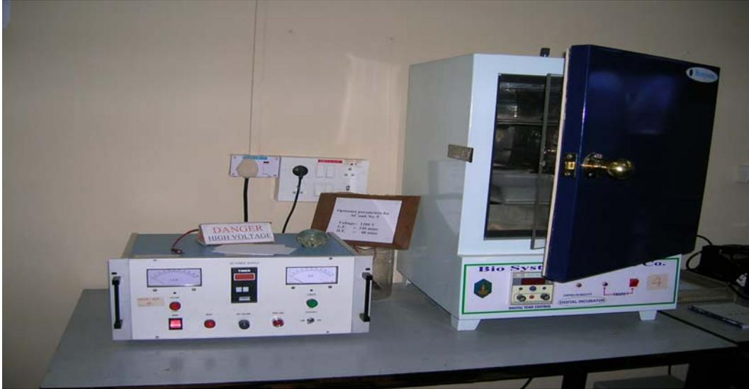
**Fig 5.** Photograph of HV power supply and incubator maintained at 60°C- for ECE.
