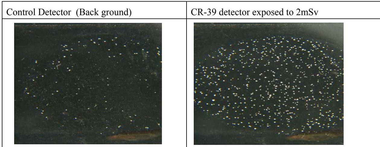
**Fig. 7:** Image of tracks on CR-39 detector after ECE processing as seen through image analysis system.
