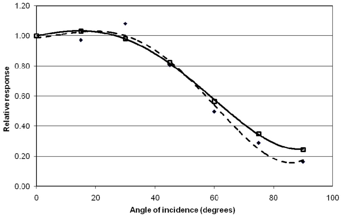
**Fig.14:** Directional dependence CR-39 dosimeter for  $^{252}\text{Cf}$  (*dashed line*) and  $^{241}\text{Am-Be}$  (*solid line*) spectra processed by ECE Technique. The response is normalized to  $0^\circ$  (*normal incidence of neutrons to detector surface*).
