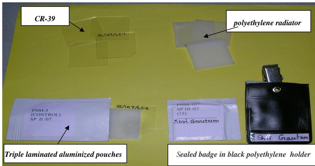
**Fig.1:** Photograph of different components of neutron badge along with the assembled badge
