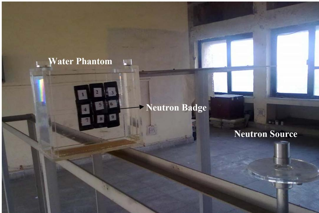
**Fig. 9:** Irradiation set-up of neutron badges for calibration.
