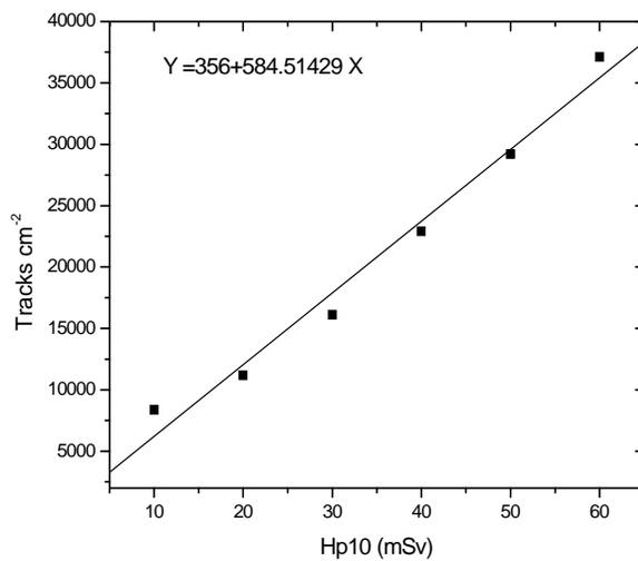
**Fig.11:** Dose linearity of CR-39 using CE technique in the dose equivalent range 10-60 mSv for <sup>241</sup>Am-Be fast neutrons. Calibration factor = 0.0016 mSv-cm<sup>2</sup> tracks<sup>-1</sup>
